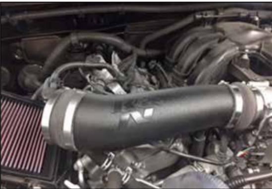
10. Install the K&N® intake tube assembly onto the throttle body as shown but do not secure at this time.
