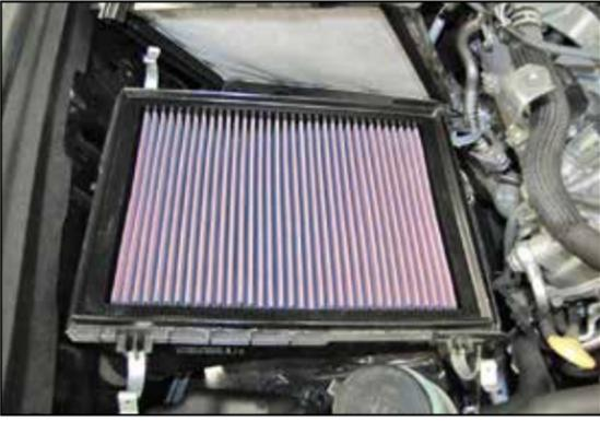
7. Remove the factory air filter and replace it with the provided K&N® air filter.
