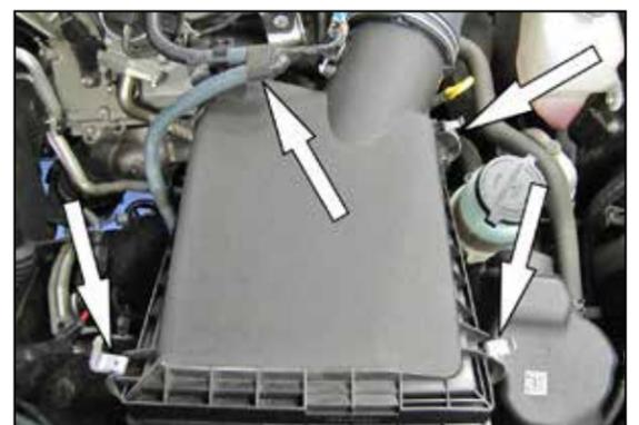
6. Release the three air filter housing clips and then lift off the upper air filter housing and remove the intake tube assembly from the vehicle.
