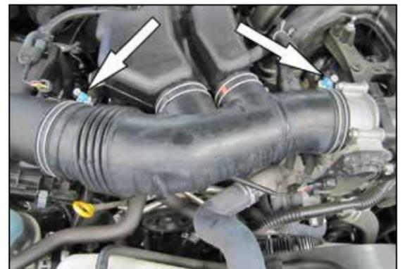
5. Loosen the two hose clamps that secure the intake tube assembly to the throttle body and air filter housing.
