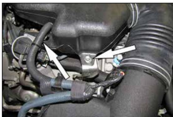
4. Remove the bolt which secures the intake plenum to the mounting bracket and unhook the mass air sensor wiring harness from the intake plenum.
