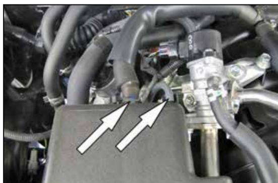
3. Release the spring clamp securing the crank case vent hose and then disconnect the crank case vent hose and the fuel pressure regulator vent hose from the factory intake tube.
