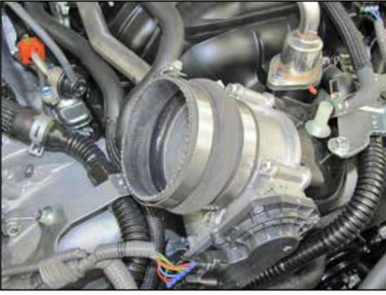
7. Install the provided coupling hose (08699) onto the throttle body and secure with the provided hose clamps as shown.
