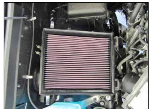
5. Release the two clips securing the factory air box lid and then remove the factory air filter. Install the provided K&N® air filter into the air box, set the air box lid into position but do not secure at this time.
