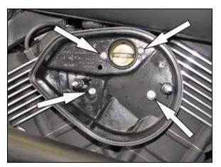
4. Remove the two throttle body bolts and the two filter back plate mounting bolts shown. NOTE: The two throttle body bolts will be reused in a later step.
