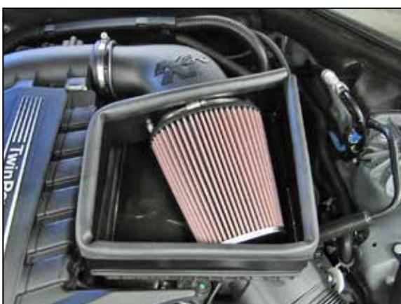
8. Install the K&N® air filter onto the intake tube and secure with the provided hose clamp.
