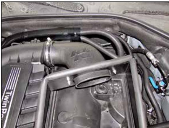
7. Install the K&N® intake tube assembly into the heat shield and intake tube as shown. Secure the intake tube with the provided hardware and the factory hose clamp.
