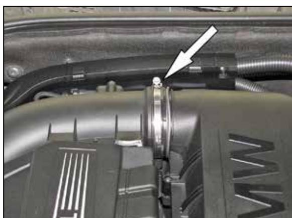
2. Loosen the hose clamp securing the upper air filter housing to the intake tube.
