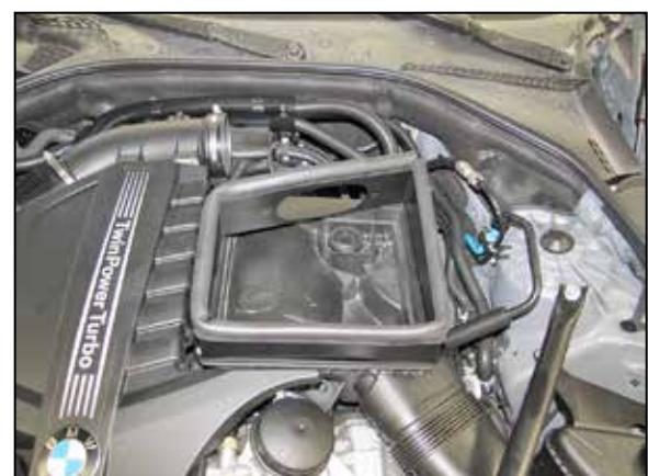
5. Install the heat shield assembly onto the lower air filter housing and secure with the provided mounting screws.
