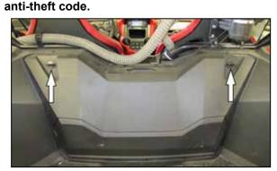
2. Unlock the two quarter turn fasteners and then remove the air filter access panel.
