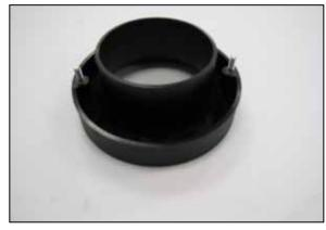
18. Install the two provided studs into the filter adapter as shown.
