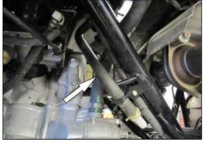
6. Remove the air filter housing drain hose shown.
