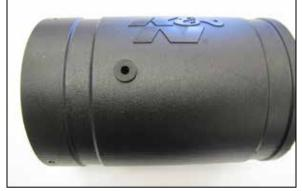
15. Drill an 11/16"id hole at the marked location and install the provided grommet into the housing. NOTE: The hole should be in the approximate location shown in the photo.
