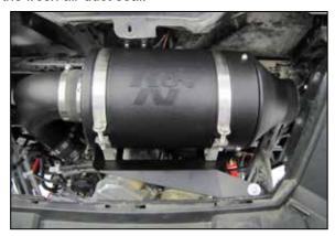
23. Install the K&N air filter assembly along with the provided large hump coupler. Secure the housing with the clamps and secure the coupler with the hose clamps.
