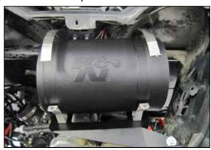
14. Place the K&N air filter housing into position on the clamps, using the factory inlet air temperature sensor wiring harness as a guide mark the housing for a drill point.
