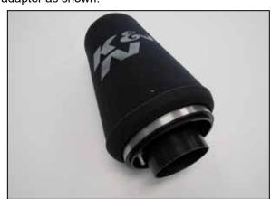
19. Install the K&N air filter onto the filter adapter and secure with the provided hose clamp, then install the foam filter wrap onto the air filter.
