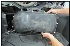
9. Partially remove the air filter system and then disconnect the inlet air temperature sensor electrical connection. Now remove the air filter assembly completely from the vehicle.
