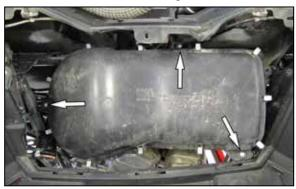
7. Remove the three bolts that secure the air filter housing.
