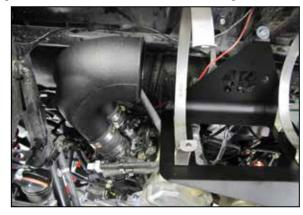
17. Install the K&N intake tube into the couplers at the throttle bodies and secure with the provided hose clamps. Connect the CCV hose to the fitting installed into the K&N intake tube and secure with the provided clamp.
