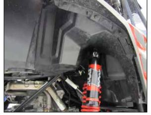
3. Remove the 12 clips that secure the fresh air duct cover and then remove the cover.
