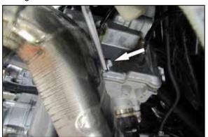
8. Remove the bolt that secures the air filter housing bracket to the exhaust.
