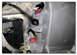
22. Remove the retaining clips and then remove the fresh air duct seal.
