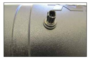
16. Remove the inlet air temperature sensor from the factory air filter housing and install it into the grommet installed into the K&N housing.
