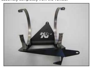
10. Install the two provided canister mounting bracket clamps onto the mounting bracket.
