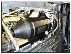
30. Install the filter housing assembly into position using just the upper mounting bolts, do not tighten the bolts.
