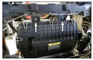
6. Remove the two bolts that secure the air filter housing to the chassis and then remove the housing from the vehicle.
