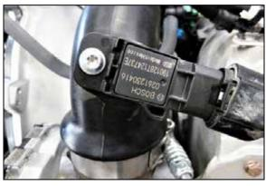
13. Remove the bolt that secures the charge pipe sensor and then remove the sensor from the vehicle.
