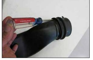
33a. On 2021 and later models it will be necessary to remove the complete fresh air supply duct fro, the vehicle and then remove the coupler adhered to the duct using a knife or screwdriver. It may also be helpful to use a heat gun.
