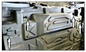
4. Slide the driver's seat forward to access the rear engine panel. Release the four quarter turn fasteners and then remove the access panel.
