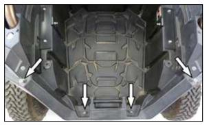
2. Remove the four bolts that secure the cargo box and then remove the cargo box from the vehicle.
