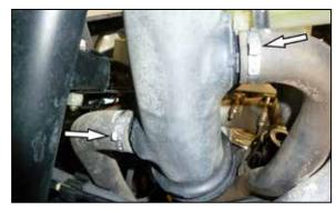
11. Loosen the two one-time use clamps that secure the vent hoses connected to the intake tube. Then disconnect the vent tubes from the intake tube and remove the intake tube from the vehicle.
