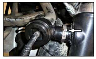
12.Loosen the one-time use clamp that secures the BOV to the charge pipe and then seperate the BOV from the charge pipe.
