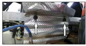
8. Remove the two heat shield bolts shown.
