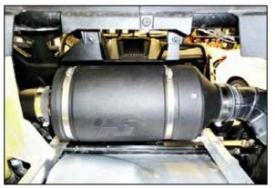
33. Install the fresh air intake duct onto the housing inlet and secure with the provided hose clamp. Note: for 2021 and later models, see steps 33a. through 33c.
