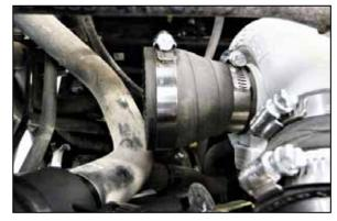
20. Install the provided step coupler onto the turbo inlet and secure with the provided hose clamp.
