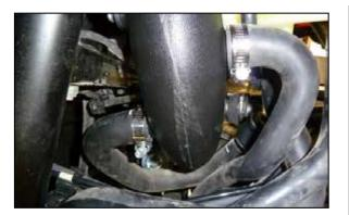
36. Install the vent lines onto the intake tube and secure with the provided hose clamps.
