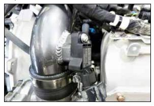
18. Install the Charge pipe sensor into the K&N charge pipe and secure with the provided hardware. Reconnect the electrical connection.
