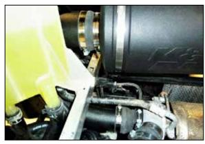
31. Install the intake tube into the coupler on the housing, align for best fit and then tighten both hose clamps.
