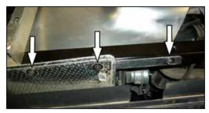
7. Remove the three bolts shown that secure the heat shield.
