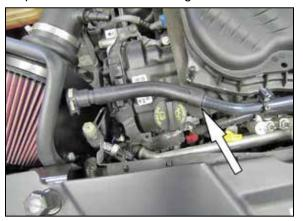
18. Remove the flexible crank case vent line from the hard line.
