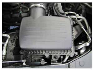
4. Pull up the factory air filter housing to dislodge it from the mounting grommets and then remove the complete intake assembly from the vehicle.
