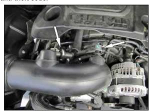
2. Disconnect the crank case vent line quick disconnect fitting. Disconnect the inlet air temperature sensor electrical connection.
