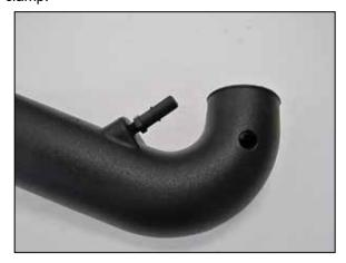
11. Install the provided NPT quick disconnect fitting into the K&N® intake tube as shown.
