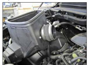
10. Install the provided hump coupler (08418) onto the filter adapter and secure with the provided hose
