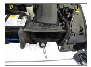
5. Remove the bolt that secures the fresh air duct to the fender. Remove the complete intake system from the vehicle.
