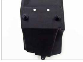
11. Install the provided mounting post onto the K&N<sup>®</sup> air filter housing using the provided hardware.
