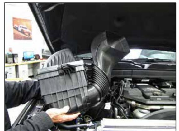
5. Remove the complete air filter housing from the vehicle as shown.
