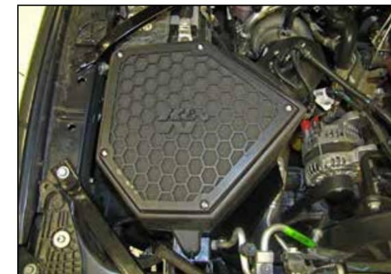
16. Assemble the prefilter lid as shown and then install onto the K&N® air filter housing and secure with the provided hardware.
