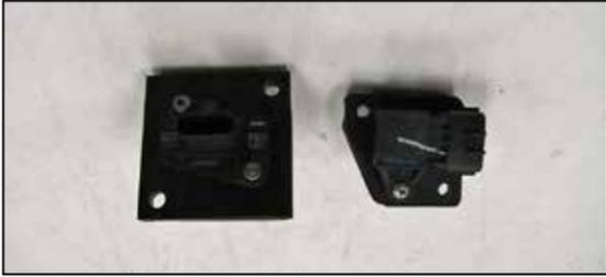
8. Remove the air sensors from the factory housing and install them into the K&N® sensor adapters using the provided hardware.
