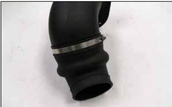
10. Install the flex coupler onto the intake tube and secure with the provided hose clamp. The coupler is keyed and can only be installed in one location.
