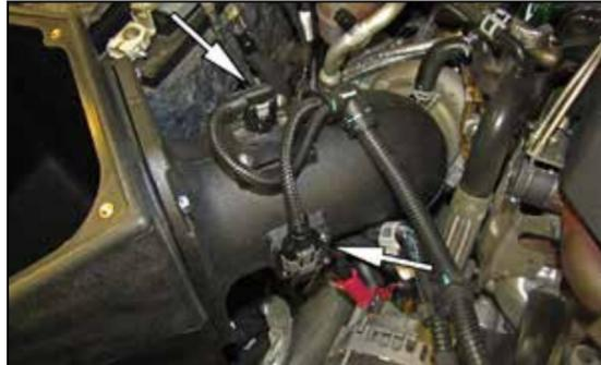
14. Reconnect the air sensor electrical connections.
