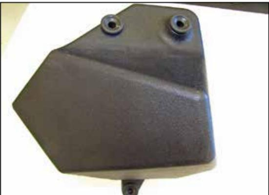
11. Remove the mounting grommets from the factory air filter housing and install them into the K&N® filter housing as shown.
