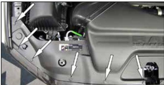
2. Remove the 14 push clips that secure the upper core support plastic cover and then remove the cover from the vehicle.
