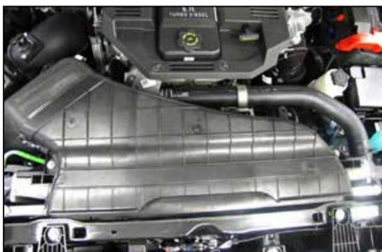
17. Install the K&N® fresh air intake duct and then install the factory upper portion of the fresh air intake duct and secure with the factory hardware.
