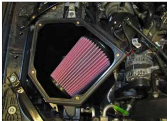
15. Install the K&N® air filter onto the intake tube and secure with the provided hose clamp.
