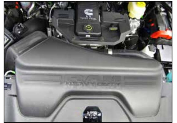
18. Reinstall the factory core support cover and secure with the factory retaining clips.
