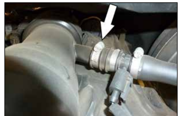
5. Loosen the hose clamp that secures the PCV hose to the factory intake tube and then disconnect the PCV hose from the intake tube.
