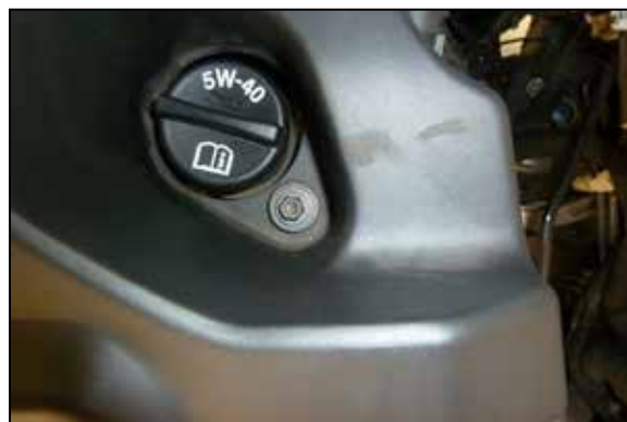
3. Remove the engine cover bolt next to the oil fill cap.
