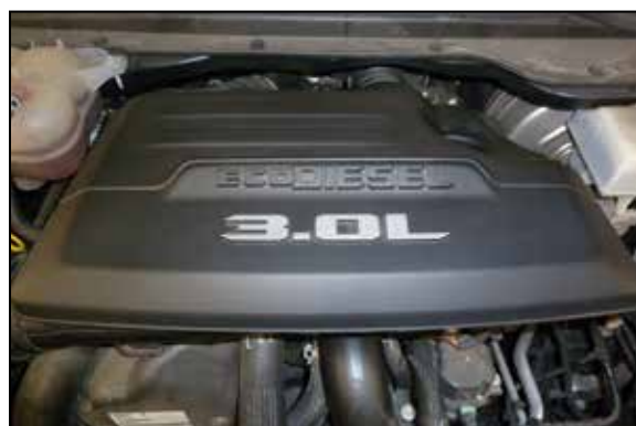
4. Pull the engine cover up, forward and then off the engine.
