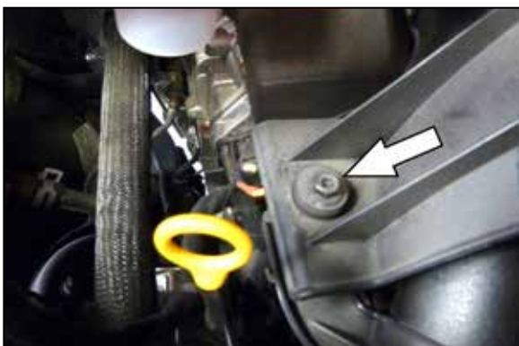
2. Remove the bolt that secures the passenger side of the engine cover.
