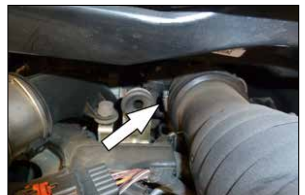
6. Loosen the hose clamp that secures the factory intake tube to the turbo inlet.
