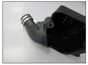
9. Install the K&N intake tube into the K&N air filter housing and secure with the provided hardware.
