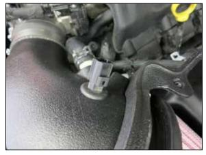
13. Remove the IAT sensor from the factory air filter housing, remove the O-ring from the sensor and then install it into the grommet installed into the K&N intake tube.
