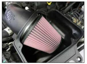
11. Install the K&N air filter onto the intake tube and secure with the provided hose clamp.
