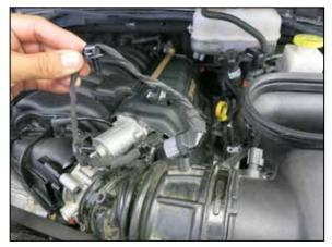
2. Disconnect the IAT sensor electrical connection and unhook the wiring harness from the intake tube.
