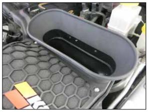
17. Install the fresh air intake seal onto the air filter housing and secure with the provided push pins.
