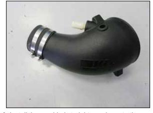
8. Install the provided straight coupler onto the K&N intake tube and secure with the provided hose clamp.
