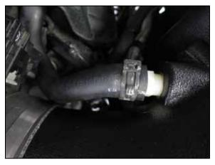
12. Connect the factory CCV hose to the fitting installed into the K&N intake.
