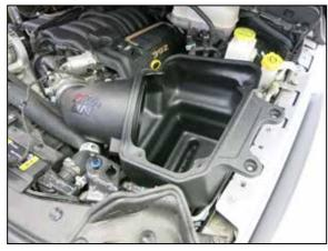
10. Set the K&N intake system into position so the coupler engages the throttle body and the posts on the bottom of the filter housing engage the factory mounting grommets. Secure the filter housing to the inner fender with the provided hardware.
