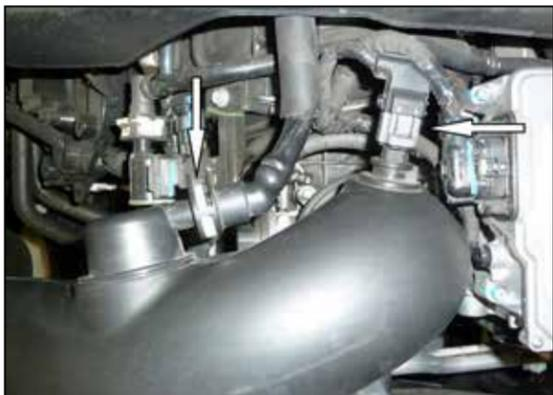
2. Disconnect the CCV quick connector and the IAT electrical connection.
