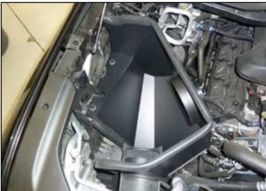
10. Install the K&N heat shield into the vehicle and secure with the factory bolt removed in the previous step. **NOTE: The upper rear tap will go between the inner fender and the air filter housing mounting bracket.**
