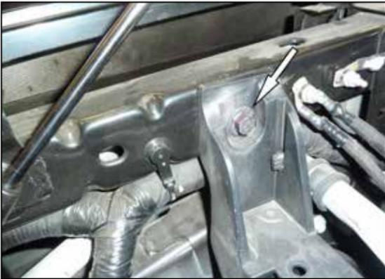
9. Remove the air filter housing mounting bracket bolt shown.
