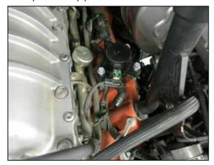
16. Reinstall the CCV switch onto the valve cover and secure with the factory bolts. Reconnect the CCV hose quick connector and connect the electrical connection.
