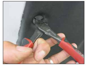
18. Cut the retaining clips that secure the left and right-side hood insulation panels. **NOTE: The clips will be destroyed during these process, new clips are provided to reinstall the insulation panels.**
