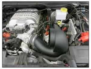
24. Install the K&N intake tube into the coupler at the throttle body but do not tighten the hose clamp to secure the tube.
