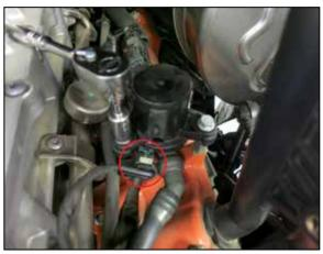
12. Disconnect the CCV switch electrical connection. Remove the mounting bolts that secure the CCV switch to the valve cover.
