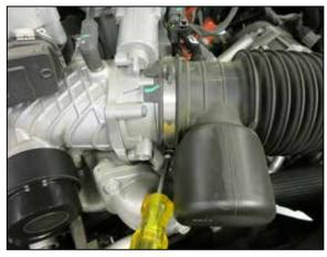
11. Loosen the hose clamp that secures the intake tube to the throttle body.
