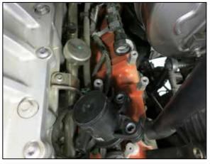
13. Disconnect the CCV line from the CCV switch at the quick connector.
