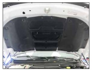
46. Reinstall the under hood insulation and secure with the provided retaining clips.
