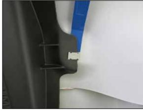
20. Using a panel popper tool or similar device, pry the clips that attach the fresh air duct to the hood to separate the duct from the hood. Remove the factory fresh air duct from the hood.
