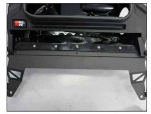
30. Secure the top side of the filter housing to the support bracket with the provided hardware.
