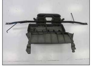
9. Remove the lower air filter housing and mounting bracket as an assembly.
