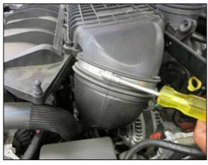
5. Loosen the hose clamp that secures the intake hose to the air filter housing.
