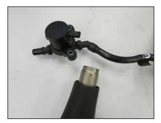
15. Using a heat gun or hair dryer, warm the connection of the CCV pipe to the CCV switch and then separate the pipe from the switch.
