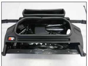
27. Install the provided edge trim onto the K&N air filter bousing
