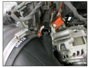
25. Connect the CCV quick connect fitting to the fitting installed into the K&N intake tube.
