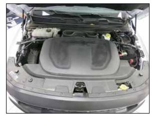
2. Unsnap the air filter housing cover and lift off.
