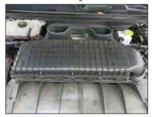
6. Loosen the ten screws that secure the upper air filter housing to the lower air filter housing and then remove the upper housing. Remove the air filters from the lower housing.
