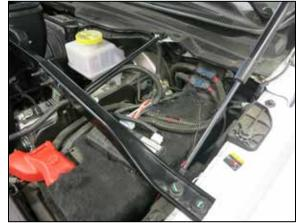
34. Secure the air filter support bracket onto the inner fenders using the factory hardware.
