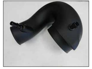
21. Remove the IAT sensor from the factory intake tube and install it into the K&N intake tube using the provided grommet. Install the provided quick connect fitting into the K&N intake tube as shown. **NOTES: The IAT sensor is fragile, use care** when handling the sensor so as not to break it. The quick connect fitting npt tapered threads and will not tighten all the way down.
