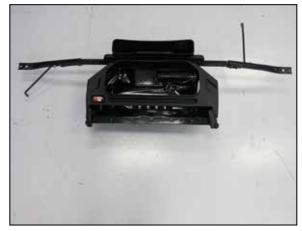
26. Secure the factory air filter housing support bracket to the K&N air filter housing using the provided hardware. Install the K&N logo into the filter housing.
