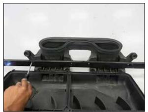
17. Remove the bolts that secure the air filter housing support bracket to the housing and set the support bracket aside.
