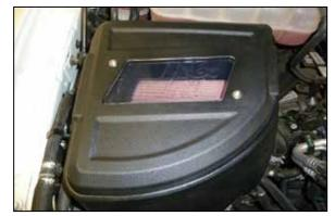
11. Install the Lid onto the filter housing so the mounting pins insert into the grommets.
