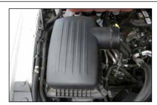
5. Lift the air filter housing assembly up and remove it from the vehicle.
