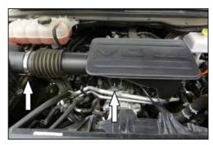
4. Loosen the hose clamp that secures the factory intake tube to the air filter housing and then remove the nut that secures the intake plenum to the intake manifold. Remove the intake plenum assembly from the vehicle.
