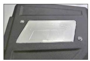
10. Install the K&N clear logo plate into the K&N filter housing lid and secure with the provided hardware.
