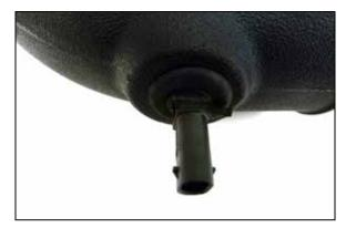
15. Remove the IAT sensor from the factory plenum, remove the O-ring from the sensor and then install the sensor into the K&N intake tube using the provided grommet.
