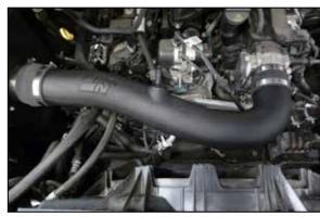
16. Install the K&N intake tube assembly into the couplers, align for best fit and then secure with the provided hose clamp.
