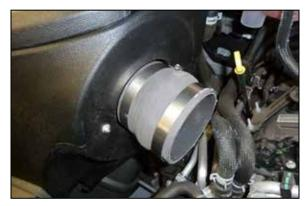
12. Install the provided hump coupler onto the filter adapter and secure with the provided hose clamp.
