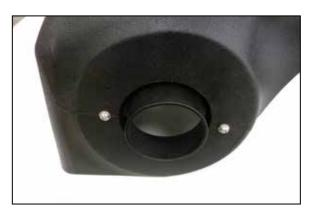
6. Install the provided radiused filter adapter into the K&N air filter housing and secure with the provided hardware.
