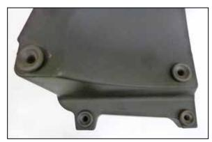
7. Remove the four mounting grommets from the factory air filter housing and then install them into the K&N air filter housing.
