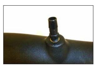
14. Install the provided vent fitting into the K&N intake tube.
