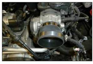
13. Install the provided step coupler onto the throttle body and secure with the provided hose clamp.
