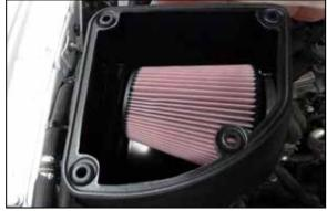
9. Install the K&N air filter onto the adapter and secure with the provided hose clamp. Install the four provided grommets into the air filter housing.
