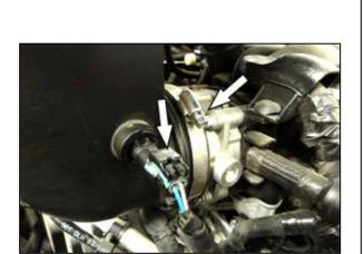
2. Loosen the hose clamp that secures the factory intake tube to the throttle body. Disconnect the IAT sensor electrical connection.
