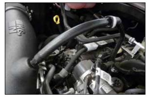
18. Install the provided CCV hose and quick connect fitting as shown
