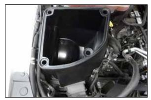
8. Set the K&N air filter housing into the vehicle so the factory mounting pins insert into the mounting grommets installed into the K&N filter housing.
