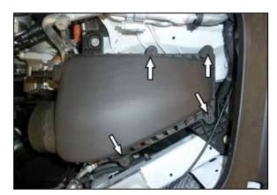
7. Remove the four bolts that secure the upper air filter housing and then remove the upper housing from the vehicle.
