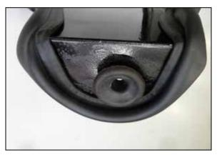
10. Remove the factory air filter housing mounting grommet and then install it into the K&N heat shield as shown.
