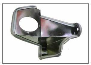
9. Install the provided edge trim onto the heat shield as shown. Some trimming of the edge trim will be necessary.
