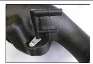
13. Install the provided O-ring onto the K&N Ejector fitting then install the fitting into the K&N intake tube and secure with the provided mounting clip and hardware.
