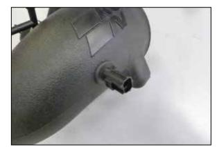
14. Remove the IAT sensor from the factory intake hose and install it into the K&N intake tube with the provided grommet.
