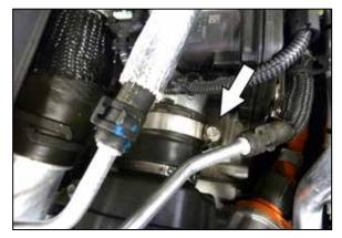
5. Loosen the hose clamp the secures the intake hose to the turbo inlet and then remove the hose from the vehicle.
