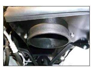
16. Secure the tube to the heat shield with the provided hardware and tighten the hose clamp at the coupler.
