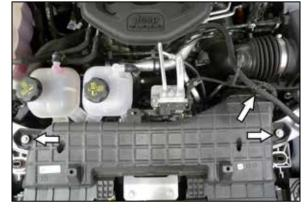
3. Unhook the wiring harness from the fresh air duct. Remove the two bolts that secure the fresh air duct then remove the fresh air duct from the vehicle.
