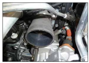
12. Install the step coupler onto the turbo inlet and secure with the provided hose clamp.
