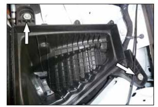
8. Remove the two bolts that secure the lower air filter housing and then remove the housing from the vehicle.
