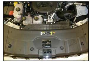
20. Reinstall the valence and secure the factory push pins.
