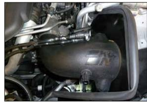
15. Install the K&N intake tube into the heat shield and coupler.
