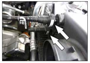
6. Push in the locking tabs and then disconnect the Ejector lines from the intake plenum.
