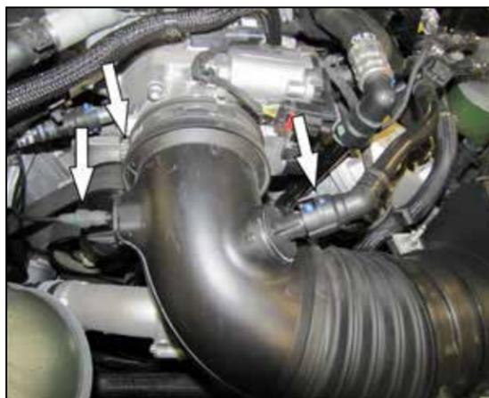
3. Disconnect the two vent lines attached to the factory intake tube. Loosen the hose clamp that secures the intake tube to the throttle body.
