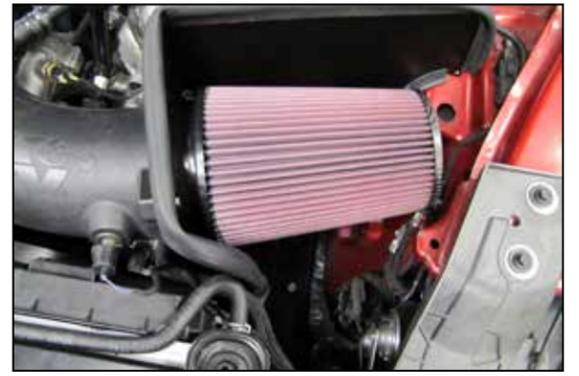
17. Install the K&N air filter and secure with the provided hose clamp.
