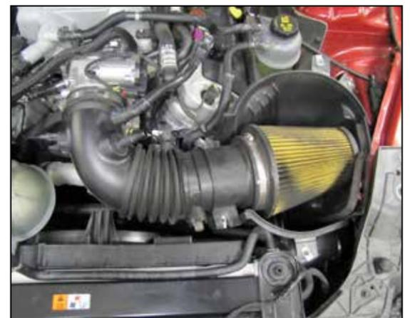
5. Remove the intake tube and filter assembly from the vehicle.
