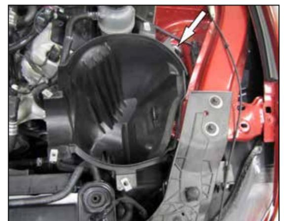
6. Remove the bolt that secures the factory air box to the inner fender and then remove it from the vehicle.
