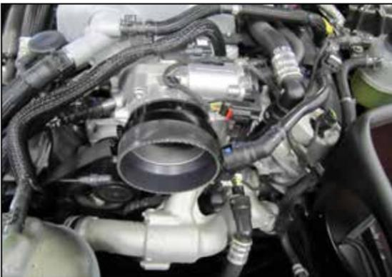
11. Install the provided coupler onto the throttle body and secure with the provided hose clamp.
