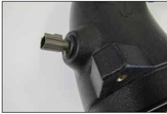
12. Remove the IAT sensor from the factory intake tube and install it into the K&N intake tube using the provided grommet.
