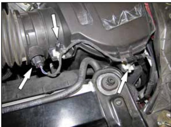
2. Disconnect the IAT sensor electrical connection and unhook the wiring harness from the air filter housing.
