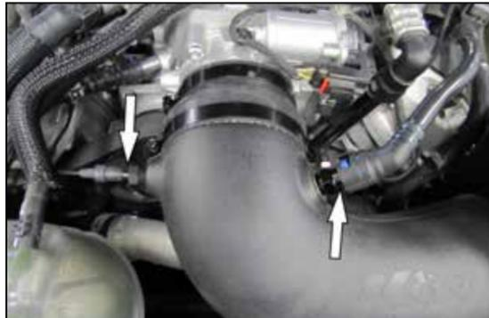
15. Connect the two factory vent lines to the fittings installed into the K&N intake tube.
