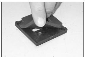
17. Install the provided gasket to the back of the K&N $^{\mbox{\tiny B}}$  mass air sensor adaptor plate as shown.
