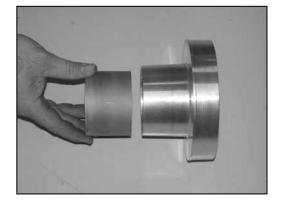
22. Vehicles that come equipped with Hydracarbon trap, place the Hydrocarbon trap into the filter adapter as shown.
