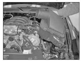
6. Remove the air box assembly as shown. NOTE: K&N Engineering, Inc., recommends that customers do not discard factory air intake.
