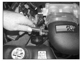
20. Install the supplied vent hose onto the vent port on the valve cover and secure with the provided hose clamp, then onto the K&N<sup>®</sup> intake tube as shown.
