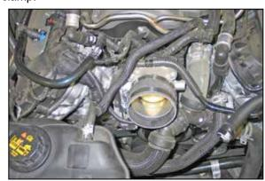
19. Install the provided silicone hose (08698) onto the throttle body and secure with the provided hose clamp.
