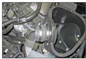
18. Install the provided silicone hose (08418) onto the filter adapter and secure with the provided hose clamp.
