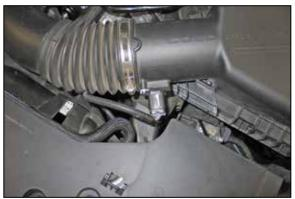
6. Unhook the mass air sensor electrical connection.
