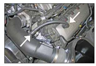
27. Install the crankcase vent hose to the fitting on the K&N® intake tube and onto the valve cover. Vehicles equipped with an EVAP vent line, connect it to the fitting installed in the K&N® intake tube.
