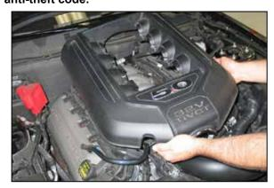
2. Lift up the engine cover and remove it from the vehicle.
