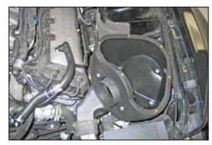
17. Set the K&N<sup>®</sup> airbox into the vehicle so that the mounting studs slide into the mounting holes, and then secure with the hardware provided.
