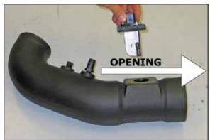
25. Install the mass air sensor assembly into intake tube and secure with the provided hardware. NOTE: Be sure the open end of the sensor is facing the filter end of the tube.
