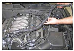
4. Release the clamp which secures engine pulse hose to the intake tube then remove the engine pulse hose from the vehicle.
