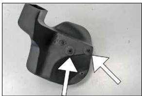
16. Install the airbox mounting grommets onto the two mounting studs installed on the K&N® airbox.
