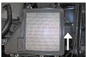
11. Remove the bolt that secures the lower airbox to the inner fender.
