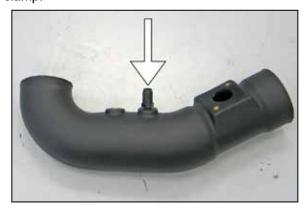
20. Install the crankcase vent fitting into the  $K\&N^{\circledcirc}$  intake tube as shown.
