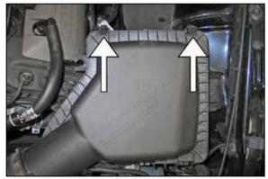
9. Release the two upper airbox retaining clips.
