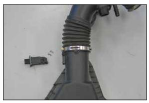
22. Remove the two bolts securing the mass air sensor into the factory intake tube and then remove the mass air sensor from the intake tube.
