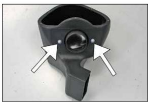
14. Install the filter adapter into the airbox and secure with the provided hardware.
