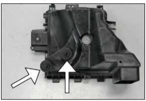
15. Remove the two airbox mounting grommets from the factory airbox.
