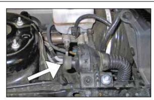
5. Install the provided cap onto the drum as shown.
