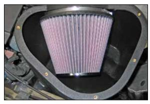
29. Install the K&N® air filter onto the filter adapter and secure with the provided hose clamp. NOTE: Drycharger® air filter wrap; part # RF-1036DK is available to purchase separately. To learn more about Drycharger® filter wraps or look up color availability please visit http://www.knfilters.com®.
