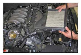
12. Remove the lower airbox from the vehicle. NOTE: K&N Engineering, Inc., recommends that customers do not discard factory air intake.
