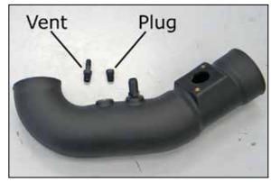
21. On vehicles that have an EVAP vent line attached to the intake tube, install the 3/8" vent fitting into the K&N® intake tube. On vehicles that do not have the EVAP vent line attached to the intake tube, install the NPT plug into the intake tube.
