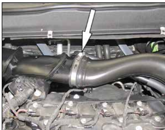
4. Loosen the hose clamp securing the intake tube to the turbo inlet.
