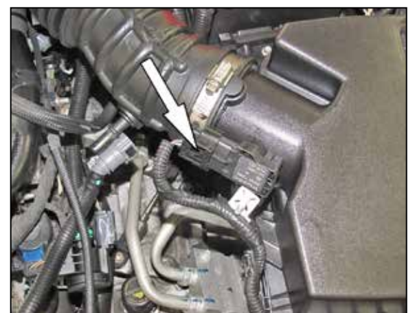
5. Disconnect the inlet air temperature sensor electrical connection then unhook the wiring harness from the upper air box housing.
