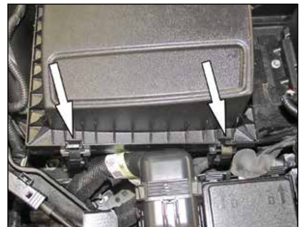
6. Release the two clips securing the upper air box to the lower air box.
