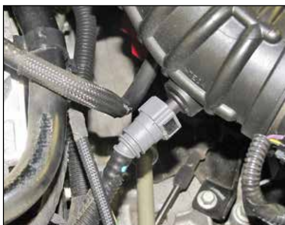
3. Disconnect the EVAP vent line by depressing the square locking tab.
