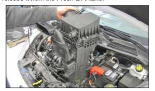
7. Remove the complete air box assembly from the vehicle by pulling up to release it from the grommets.
