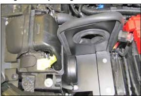
14. Reinstall the fresh air intake duct onto the core support duct as shown.
