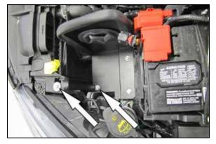
12. Secure the heat shield mounting bracket (064317) to the heat shield and core support as shown using the provided hardware.
