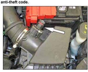
2. Release the red locking tab and then disconnect the Mass air sensor electrical connection.
