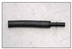
22. On 2014-15 model year vehicles, install the provided EVAP vent hose onto the provided guick disconnect union as shown.
