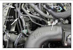
25. Install the new EVAP hose assembly to the factory fittings and the vent fitting on the K&N® intake tube. This assembly will replace the complete vent assembly removed in step #4a.
