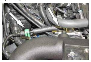
23. Install the EVAP hose assembly into the factory quick disconnect fitting and then onto the 90° fitting installed into the K&N® intake tube as shown.
