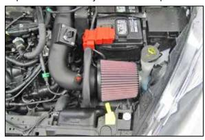
26. Install the K&N® air filter onto the intake tube and secure with the provided hose clamp. NOTE: Drycharger® air filter wrap; part # RX-4990DK is available to purchase separately. To learn more about Drycharger® filter wraps or look up color availability please visit http://www.knfilters.com®.
