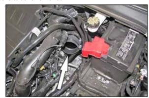
8. Install the provided hump hose (087121) onto the turbo inlet and secure with the provided hose clamp.
