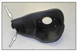
10. Install the provided edge trim around the heat shield as shown.
