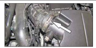
4. Loosen the hose clamp securing the factory intake tube to the air box housing.
