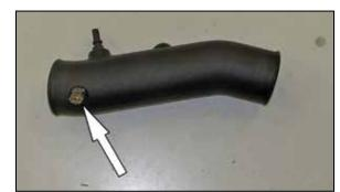
Install the provided grommet into the K&N® tube then install the inlet air temperature sensor into the grommet.
