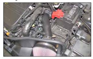
21. Install the K&N® intake tube assembly into the coupling hose at the turbo inlet and then into the coupling hose at the filter adapter. Adjust the tube for best fit and then secure with the provided clamps.
