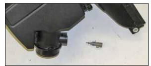
19. Remove the inlet air temperature sensor from the factory air box and remove the O-Ring from the
