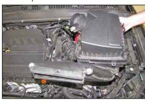
6. Lift up the air box to dislodge it from the mounting grommets and then remove it from the vehicle.
