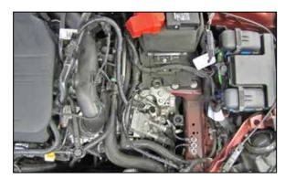
9. On 2008 and later model vehicles with the pressure sensor, connect the provided Inlet air temperature sensor extension harness to the open connector for the sensor. Then route the wiring harness along the hoses and reconnect the pressure sensor electrical connection.
