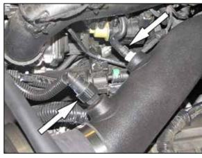
22. Connect the factory solenoid vent hose and the factory crank case vent hose to the fittings installed into the K&N® intake tube.
