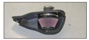
15. Install the K&N® air filter onto the filter adapter and secure with the provided hose clamp.
