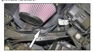
17. Clip the inlet air temperature sensor harness into the hole provided in the heat shield.
