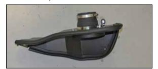
14. Install the provided step coupler (084055) onto the filter adapter and secure with the provided hose
