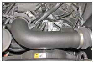
24. Install the K&N<sup>®</sup> intake tube into the hose at the filter adapter and then into the hose at the throttle body, adjust the tube for best fit and then secure with the provided hose clamps.
