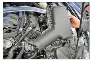
9. Remove the bolt securing the air filter assembly onto the inner fender and then air filter assembly from the engine compartment.
