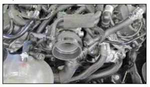
18. Install the provided hump coupler (08699) onto the throttle body and secure with the provided hose clamp.  $K\&N^{\circ}$  intake tube so that the opening in the sensor faces towards the filter end of the tube and secure with the provided hardware.
