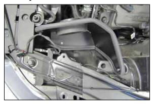
14. Set the heat shield onto the mounting bracket installed in step #9 and secure with the provided hardware.
