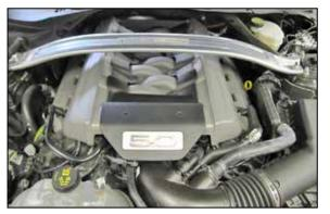
2. Lift up the decorative engine cover to dislodge it from the mounting studs and then remove the engine cover from the vehicle.
