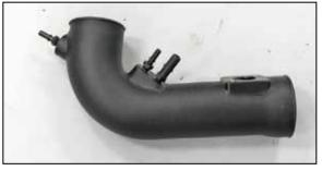
19. Install the quick disconnect fittings into the  $K\&N^{\circledast}$  intake tube as shown.
