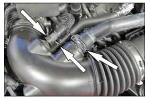
4. Depress the locking tabs and then disconnect the crank case vent hose and the EVAP vent hose. Then release the spring clamp and disconnect the sound tube from the intake tube. NOTE: Some vehicles are not equipped with the
