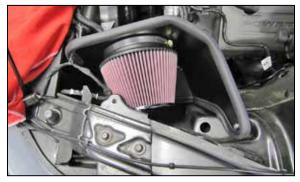
15. Install the K&N<sup>®</sup> air filter onto the adapter and secure with the provided hose clamp.
