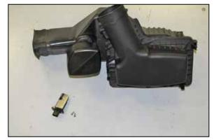
21. Remove the mass air sensor from the factory air filter housing.
