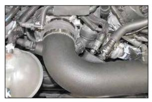
25. Connect the crank case vent, EVAP vent and idle by pass lines to the quick disconnect fittings installed into the K&N<sup>®</sup> intake tube.
