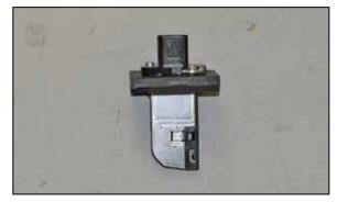
22. Install the mass air sensor into the adapter and secure with the provided hardware.
