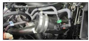
14. Install the provided coupling hose (08761) onto the driver's side turbo inlet tube and secure with the provided hose clamp.
