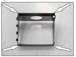
8. Install the small edge trim onto the heat shield as shown using the provided super glue to secure.
