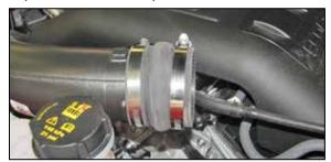
15. Install the provided coupling hose (087121) onto the passenger side turbo inlet tube and secure with the provided hose clamp.
