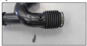
17. On vehicles equipped with an inlet temperature sensor, unlock the inlet air temperature sensor and rotate it counter clockwise, remove the sensor from the factory air filter housing.
