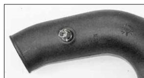
18. On vehicles equipped with an inlet temperature sensor, remove the O-Ring from the inlet air temperature sensor and then install it into the grommet installed into the K&N® intake tube. .
