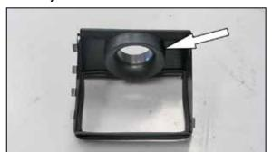
10. Install the provided filter adapter into the heat shield and secure with the provided hardware.
