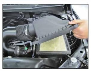
5. Lift up and remove the upper air filter housing and factory air filter.
