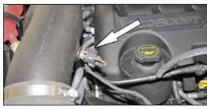
20. On vehicles equipped with an inlet temperature sensor, reconnect the inlet air temperature sensor electrical connection.
