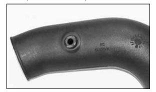
16. Install the provided grommet into the K&N® intake tube as shown.
