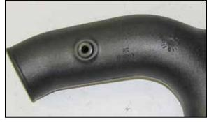
16. Install the provided grommet into the  $K\&N^{\circledast}$  intake tube as shown.
