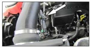
20. Reconnect the inlet air temperature sensor electrical connection.
