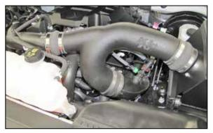
19. Install the K&N<sup>®</sup> intake tube into the turbo inlet hoses and then into the hose at the throttle body, adjust the tube for best fit and then secure with the provided hose clamps.
