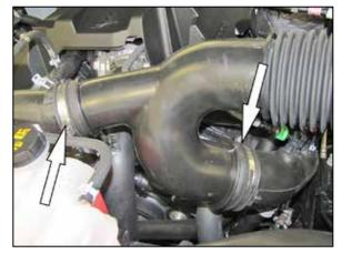
6. Loosen the hose clamps securing the intake tube to the two turbo inlet tubes and then remove the intake tube from the vehicle.
