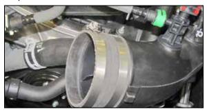
14. Install the provided coupling hose (08761) onto the driver's side turbo inlet tube and secure with the provided hose clamp.
