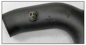
18. Remove the O-Ring from the inlet air temperature sensor, then install it into the grommet installed into the K&N<sup>®</sup> intake tube. **NOTE: The inlet air temperature sensor is very fragile, be careful while installing the sensor so as not to break it.**  NOT LEGAL FOR SALE OR USE ON ANY POLLUTION CONTROLLED MOTOR VEHICLE IN CALIFORNIA OR STATES ADOPTING CALIFORNIA EMISSION PROCEDURES.
