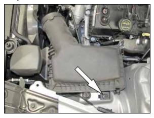
4. Remove the bolt securing the factory air filter housing and then remove the complete air filter housing from the vehicle.
