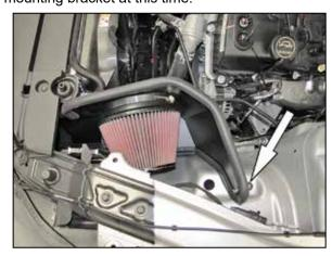
10. Flex the heat shield back and install the K&N® air filter onto the adapter then secure the filter with the hose clamp. Secure the upper heat shield mounting bracket with the hardware provided.
