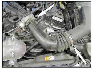
3. Loosen the hose clamps and then remove the factory intake tube.
