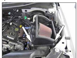
10. Install the heat shield assembly onto the lower air filter housing and secure with the factory retaining clips.
