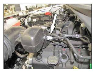
Disconnect the EVAP vent quick connect fitting.
