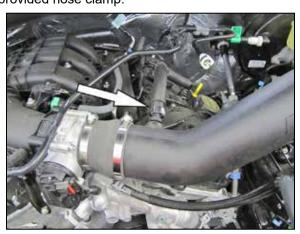
15. Connect the crank case vent quick disconnect fitting to the mating quick disconnect fitting installed into the K&N® intake tube.
