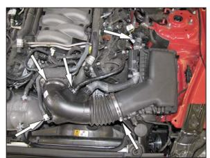
5. Release the retaining clip securing the EVAP vent lines and then disconnect the lines from the intake tube. Locate the hose clamp that secures the Sound tube to the Sound drum located on the driver side strut tower. Release the clamp by cutting with pliers and then disconnect the sound tube from the drum. Loosen the hose clamps that secure the intake tube to the throttle body and air filter housing and then remove the tube from the vehicle.
