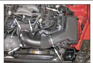
5. Release the retaining clip securing the EVAP vent lines and then disconnect the lines from the
