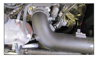
16. Connect the EVAP and crank case vent lines to the fittings installed into the K&N® intake tube.
