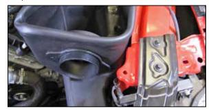
14. Install the filter adapter into the K&N<sup>®</sup> air filter housing and then install the tube gasket onto the adapter.
