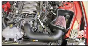
19. Unhook the mass air sensor wiring harness from the inner fender and then route to the mass air sensor and reconnect.
