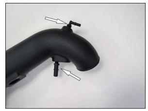
9. Install the provided fittings into the K&N $^{\! \rm B}$  intake tube as shown.
