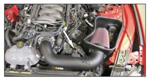
19. Unhook the mass air sensor wiring harness from the inner fender and then route to the mass air sensor and reconnect.
