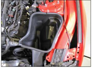
8. Install the provided edge trim onto the K&N® air filter housing. Install the K&N® air filter housing into the vehicle and secure with the provided hardware. NOTE: Some trimming of the edge trim will be necessary.
