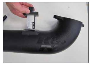
12. Install the mass air sensor assembly into the K&N<sup>®</sup> intake tube as shown and secure with the provided hardware. **NOTE: Be sure to install the maf sensor in the correct direction as shown in the photo. The vehicle will not run properly if the sensor is installed backwards.**
