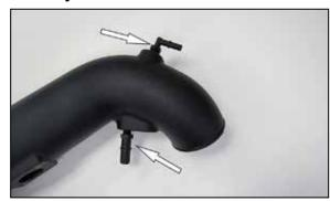
9. Install the provided fittings into the K&N<sup>®</sup> intake tube as shown. **NOTE: Plastic NPT fittings are** easy to cross thread. Install the vent fitting "hand" tight, then turn it two complete turns with a wrench.
