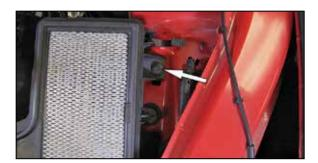
7. Remove the bolt that secures the air filter housing to the inner fender and then remove the lower air filter housing from the vehicle. **NOTE: K&N Engineering, Inc., recommends that customers do not discard factory air intake.**
