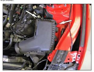
6. Release the clips that secure the upper air filter housing and then remove the upper air filter housing from the vehicle.
