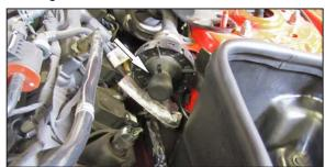
17. Install the provided cap onto the sound drum as shown.
