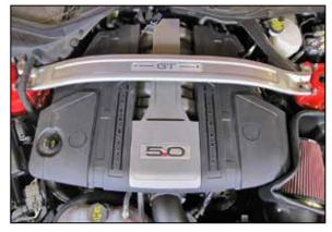
20. Reinstall the engine cover and secure with the factory hardware, reinstall the nut covers. Reinstall the strut tower brace and secure with the factory nuts.
