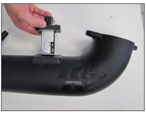
12. Install the mass air sensor assembly into the K&N® intake tube as shown and secure with the provided hardware. NOTE: Be sure to install the maf sensor in the correct direction as shown in the photo. The vehicle will not run properly if the sensor is installed backwards.
