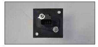
11. Remove the mass air sensor from the factory air filter housing and install it into the  $K\&N^{\mbox{\tiny ®}}$  adapter
