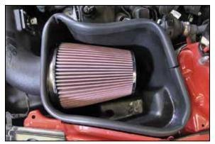
18. Install the K&N<sup>®</sup> air filter onto the filter adapter and secure with the provided hose clamp. NOTE: Drycharger<sup>®</sup> air filter wrap; part # RF-1020DK is available to purchase separately. To learn more about Drycharger<sup>®</sup> filter wraps or look up color availability please visit http://www.knfilters.com<sup>®</sup>. NOT LEGAL FOR SALE OR USE ON ANY POLLUTION CONTROLLED MOTOR VEHICLE IN CALIFORNIA OR STATES ADOPTING CALIFORNIA EMISSION PROCEDURES.
