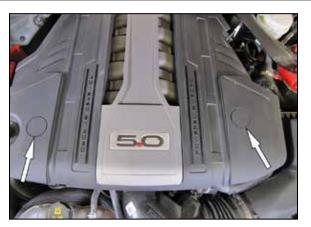
3. Remove the fastener covers on the engine
