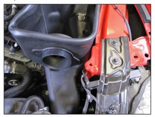
14. Install the filter adapter into the K&N® air filter housing and then install the tube gasket onto the adapter.
