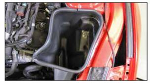
8. Install the provided edge trim onto the K&N<sup>®</sup> air filter housing. Install the K&N<sup>®</sup> air filter housing into the vehicle and secure with the provided hardware. **NOTE: Some trimming of the edge trim will be necessary.**
