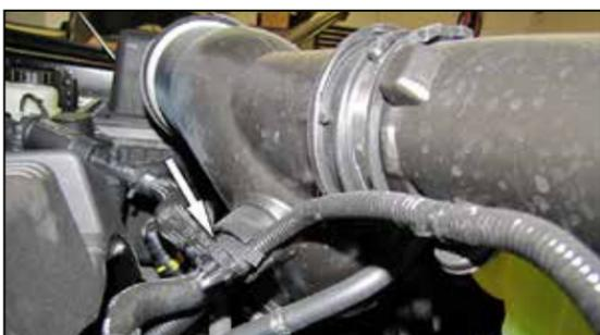
2. Disconnect the inlet air temperature sensor electrical connection.
