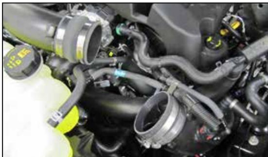
17. Install the provided hump coupler (087121) onto the upper (passenger side) turbo inlet pipe and coupler (08761) onto the lower (Drivers side) turbo inlet pipe and secure with the provided hose clamps.
