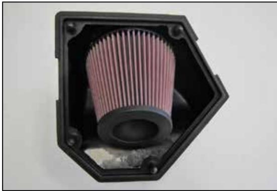
14. Install the air filter assembly into the upper air filter housing and secure with the provided hardware.
