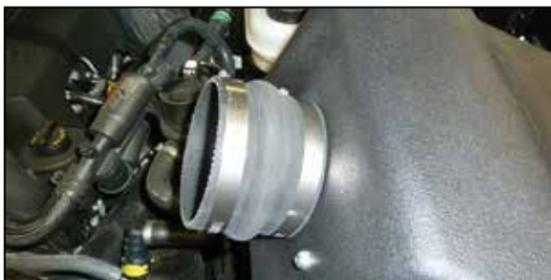
16. Install the provided hump coupler (08699) onto the filter adapter and secure with the provided hose clamp.
