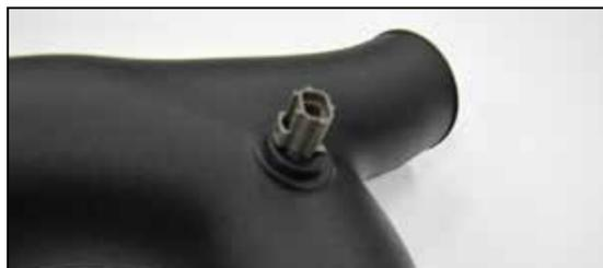
18. Remove the inlet air temperature sensor from the factory intake tube and remove the O-ring from the sensor. Using the provided grommet, install the inlet air temperature sensor into the K&N® intake tube as shown.
