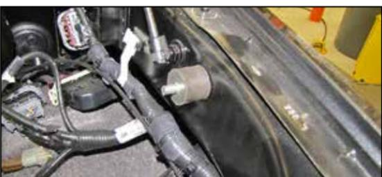
11. Install the rubber mounted stud into the factory inner fender air filter housing mounting location as shown.
