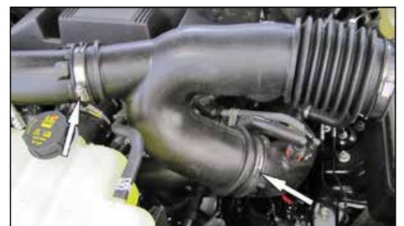
5. Loosen the two remaining hose clamps that secure the factory intake tube to the turbo inlet pipes and then remove the intake tube from the vehicle.
