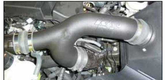
19. Install the K&N® intake tube into the couplers for the turbo inlet pipes and the filter adapter, adjust the tube for best fit and then secure with the provided hose clamps.
