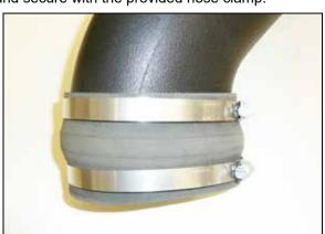
14. Slide the provided hump coupler completely onto the intake tube with the hose clamps as
