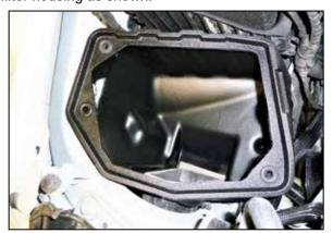
9. Install the K&N air filter housing and secure to the inner fender with one of the factory bolts from step #7.
