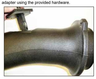
11. Install the mass sensor assembly into the K&N intake tube, be sure to install the sensor in the correct position so the opening of the sensor is pointed towards the filter end of the intake tube.
