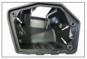
8. Install the three provided grommets into the K&N filter housing as shown.
