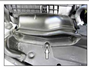
5. Remove the pin that secures the fresh air intake duct and then remove the duct from the vehicle.
