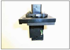
10. Install the gasket onto mass air sensor adapter and then remove the mass air sensor from the factory filter housing and install it into the K&N
