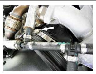
3. Loosen the hose clamp that secures the factory intake tube to the turbo inlet pipe.
