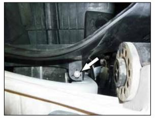
6. Remove the bolt securing the air filter housing and then remove the housing from the vehicle.
