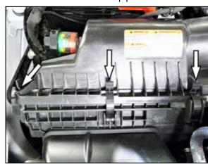
4. Release the three clips that secure the air filter housing lid and then remove the lid, intake tube and air filter from the vehicle.
