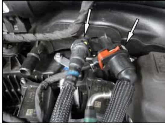
8. Release the red and yellow safety lock clips on the ejector vent lines and then release the clips that secure the ejector lines and disconnect them from the intake tube.
