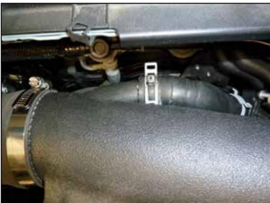
21. Connect the BOV hose to the K&N intake tube and secure with the factory spring clamp.
