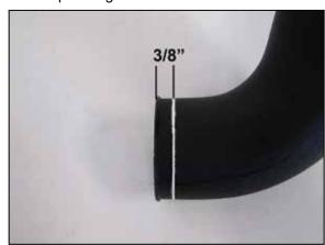
6a. On 2023 and later Ford Raptor model vehicles it is necessary to trim 3/8" off the end of tube p/n 087545. Using a marker, measure and draw a line 3/8" from the turbo inlet end of the tube as shown.
