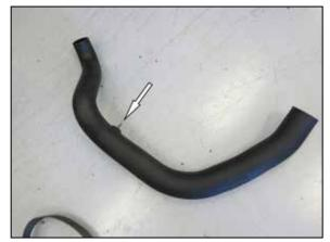
6. Install the provided 6mm stud into the insert on the K&N passenger side turbo inlet tube.
