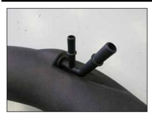
14. Install the provided ejector fitting into the K&N driver side turbo inlet tube using the provided grommet. NOTE: The ejector fitting is fragile, Grab the fitting on the main body and use a twisting motion while pushing the fitting into the grommet. Using some lubricant like WD40 will ease the installation into the grommet. Pushing in the fitting on the top vent leg may result in the fitting fracturing.
