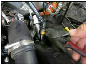
10. Using a pair of side cutters, cut the black the black hard-shell portion of the CCV connectors at the valve cover and turbo inlet tube so the fittings can be disconnected and the CCV hose assembly and be removed.
