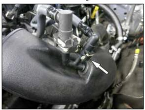
21. Connect the vent lines to the ejector fitting installed into the K&N inlet tube.
