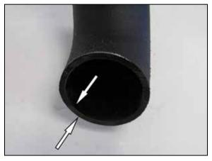
6b. Using a saw, carefully cut the tube at the line marked in the previous step. Once the tube is cut use a deburring knife or similar device to remove all burrs and cutting debris along the inside and outside edge of the tube. Carefully clean the tube of any shavings or debris before installation.
