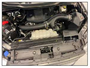
22. Reinstall the air filter housing and intake tube. NOTE: Shown with K&N intake kit 63-2617 installed.
