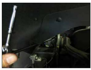
7. Place the K&N passenger side turbo inlet tube into position in the coupler and so the 6mm stud aligns with the mounting grommet. Secure the tube with the hardware and clamp provided.
