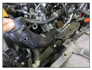
11. Loosen the hose clamp at the turbo inlet, unhook the mounting post and remove the driver side turbo inlet tube.
