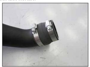
12. Install the provided step coupler and hose clamps onto the K&N driver side turbo inlet tube.
