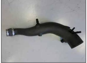
16. Assembled K&N driver side turbo inlet tube.
