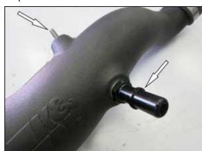
13. Install the provided CCV fitting and mounting stud into the K&N driver side turbo inlet tube.
