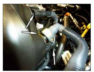
3. Depress the locking tabs and then disconnect the three vent lines attached to the driver side intake tube.
