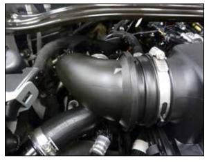
2. Loosen the hose clamps that secure the passenger side intake tube to the turbo inlet and factory air filter housing. Remove the passenger side intake tube from the vehicle.
