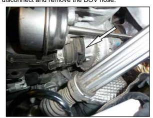
7. Release the spring clamp the secures the driver side intake tube to the turbo inlet and then remove the intake tube from the vehicle.
