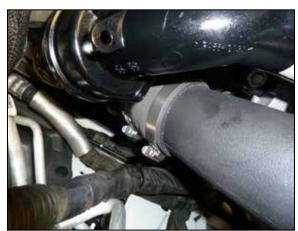
23. Install the passenger side intake tube into the coupler at the turbo inlet and into the K&N air filter housing.
