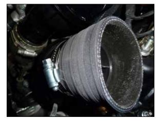
22. Install the provided coupler onto the passenger side turbo inlet.
