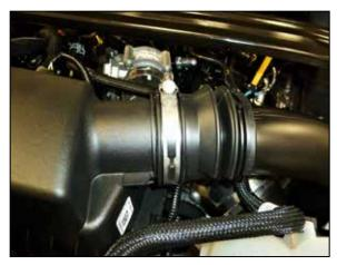
4. Loosen the hose clamps that secure the driver side intake tube to the air filter housing.
