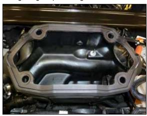
11. Install the K&N air filter housing into the vehicle and secure with the provided fender washer and factory mounting nuts.
