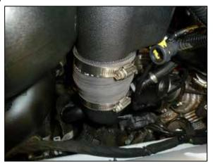
19. Install the driver side upper intake tube into the coupler on the lower intake tube and into the K&N air filter housing.
