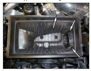
9. Remove the lower air box mounting nut. Release the three locking tabs that secure the fresh air intake duct and the unhook the duct from the lower air filter housing.
