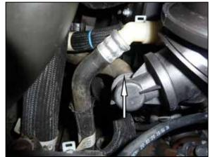
6. Release the BOV hose spring clamp and then disconnect and remove the BOV hose.
