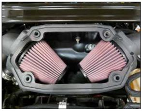
25. Install the air filters onto the intake tube and secure with the provided hose clamps. Install the four grommets into the lid mounting holes in the air
