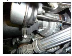
14. Install the lower driver side intake tube onto the turbo inlet and secure with the provided hose clamp.
