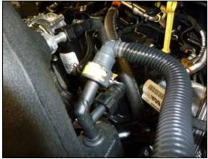
21. Connect the vent lines to the quick connect
