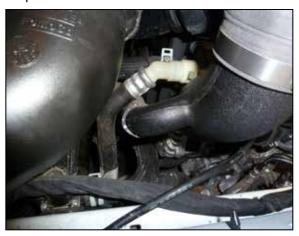
15. Connect the BOV hose to the K&N lower intake tube.
