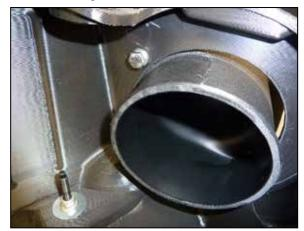
20. Secure the driver side intake tube to the air filter housing with the provided hardware then tighten all the hose clamps.
