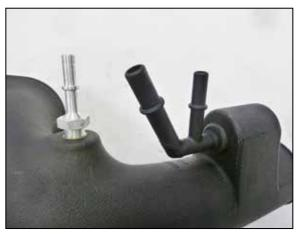
16. Install the quick connect fitting into the driver side upper K&N intake tube. Install the provided ejector fitting with the provided grommet into the intake tube. NOTE: When installing the ejector fitting, grab it on the main shaft not the extended portion to prevent possible breakage.
