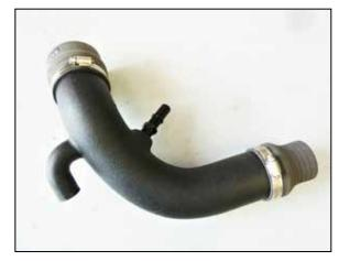
13. Install the provided couplers and quick connect fitting into the lower driver side intake tube.
