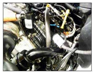
18. Connect the assembled CCV hose to the fitting installed into the intake tube and to the valve cover port.
