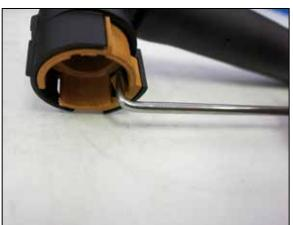
5. Disconnect the CCV hose from the valve cover. There are three clips inside the connector that lock the fitting onto the valve cover, using a 90 degree pick or similar device the clips can be released one at a time while applying slight pressure upwards on the fitting. The upward pressure will help prevent the clips from relocking while releasing the others. Replacement connectors are provided to be used with the K&N intake kit.
