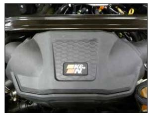
26. Install the K&N badge into the lid and then install the lid onto air filter housing.
