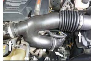
2. Loosen the three hose clamps that secure the intake tube to the air filter and turbo inlet tubes and then remove the tube from the vehicle.
