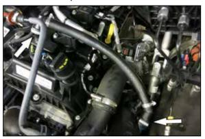
19. Remove the factory CCV hose assembly from the valve cover and install the CCV hose assembly onto the valve cover and turbo inlet tube fittings.
