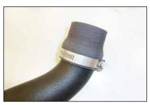
12. Install the provided step coupler and hose clamps onto the K&N driver side turbo inlet tube.
