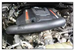
8. Place the K&N passenger side turbo inlet tube into position in the coupler and so the mounting stud aligns with the mounting grommet. Secure the tube with the hardware and clamp provided.
