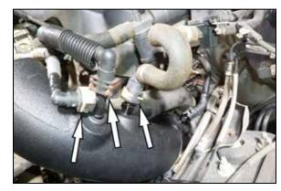
20. Connect the vent lines to the ejector fitting and CCV fittings installed into the K&N inlet tube.
