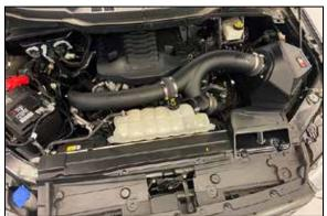
22. Reconnect the negative battery cable. Note: photo shows the inlet tubes installed along with K&N intake kit p/n 63-2617. Reconnect the vehicle's negative battery cable. Double check to make sure everything is tight and properly positioned before starting the vehicle.
