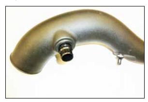
13.Install the grommet and BOV fitting into the driver side K&N turbo inlet tube. Apply a small amount of lubricant onto the fitting to ease installation.
