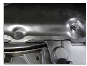
16. Install the two provided push clips to secure the fresh air duct.
