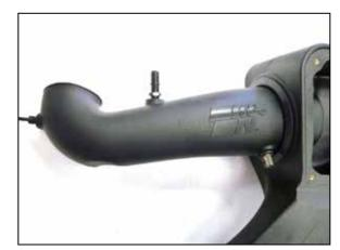
13. Install the K&N intake tube through the grommet into the air filter housing as shown.
