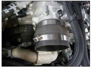
14. Install the provided step coupler onto the throttle body and secure with the provided hose clamp.
