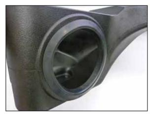
12. Install the provided tube seal grommet into the K&N air filter housing as shown.
