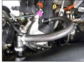
21. Install the CCV hose assembly onto the fittings on the valve cover and intake tube.
