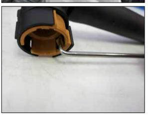
7. Disconnect the CCV hose from the valve cover. There are three clips inside the connector that lock the fitting onto the valve cover, using a 90 degree pick the clips can be released one at a time while applying slight pressure upwards on the fitting. The upwards pressure will help prevent the clips from relocking while releasing the others. Replacement connectors are provided to be used with the K&N intake kit.
