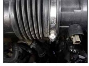
3. Loosen the hose clamp securing the intake tube to the air filter housing.
