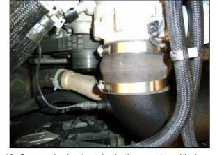
18. Secure the intake tube in the coupler with the provided hose clamp.
