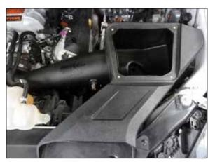
15. Install the intake assembly into the vehicle so the filter housing seats into the factory mounting grommets and the intake tube engages the coupler at the throttle body.
