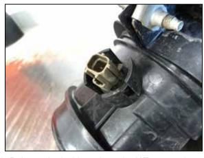
8. Release the locking tab on the IAT sensor then rotate counterclockwise and remove the sensor from the housing.
