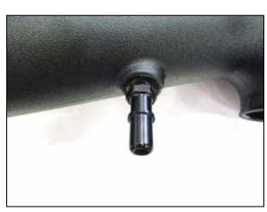
10. Install the provided quick connect fitting into the K&N intake tube as shown.
