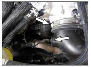
6. Disconnect the vacuum line from the intake tube then loosen the hose clamp that secures the intake tube to the throttle body.
