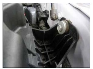
4. Remove the bolt that secures the factory air filter housing to the inner fender.
