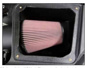
22. Install the K&N air filter onto the intake tube and secure with the provide hose clamp.
