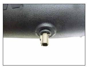
9. Remove the O-ring from IAT sensor, install the sensor into the K&N intake tube using the provided grommet.
