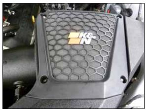
23. Assemble the pre filter lid and install it onto the air filter housing using the provided hardware.
