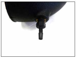
11. Install the provided vacuum fitting into the K&N intake tube as shown.
