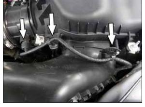
2. Disconnect the IAT sensor electrical connection and then unhook the wiring pigtail from the factory air filter housing.
