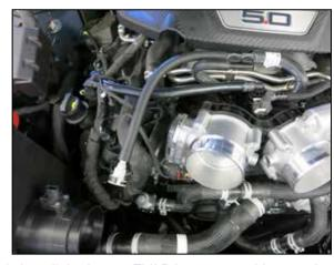
9. Install the longer EVAP hose assembly onto the check valve fitting.
