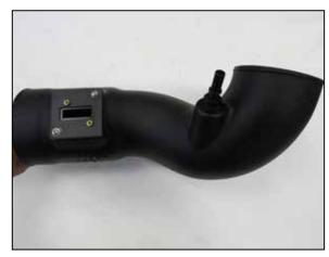
15. Passenger side tube, install the gasket to the MAF adaptor. Install the MAF adaptor to the intake tube using provided hardware. Install the 1/4" NPT quick connect to the intake tube and tighten. Note: Make sure the MAF sensor pad is installed in correct position as shown.
