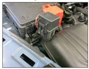
7. Pull back the relay from the fuse box assembly and set aside to allow clearance for air filter housing removal. Remove the complete passenger side intake system.
