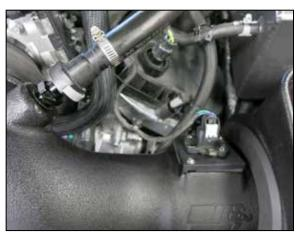
23. Reconnect the MAF sensor on the driver side and connect the crank case line.
