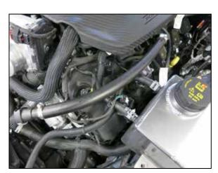
11. Disconnect the OEM plastic crank case hard line and remove from vehicle. Install the new crank case rubber line into the vehicle.
