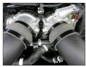
24. Secure and tighten the clamps on the throttle body.
