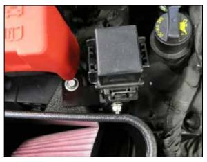
20. Secure the passenger side air box using original bolt and new relay bracket from step 13. Once tighten, secure the relay to the metal tab.
