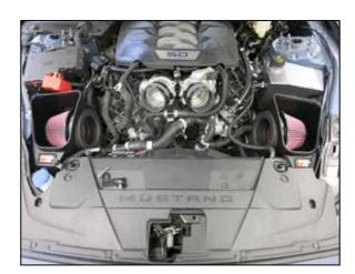
19. Install both air boxes into the vehicle and secure the driver side using original bolt.
