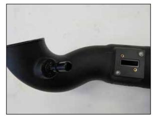
16. Driver side tube, install the gasket to the MAF adaptor. Install the MAF adaptor to the intake tube using provided hardware. Install the 3/8" NPT quick connect to the intake tube and tighten. Note: Make sure the MAF sensor pad is installed in correct position as shown.
