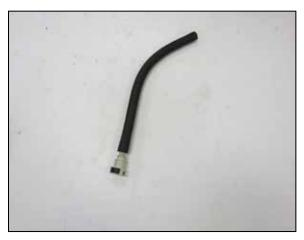
8. Remove the EVAP hose from the engine. Remove the quick connect fitting from the factory EVAP hose and install it into the provided longer EVAP hose.
