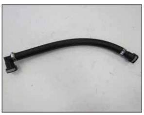
10. Assemble the new Crank case line with provided quick connect fittings and mini clamps. Secure and tighten.
