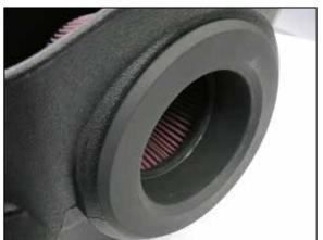
17. Install the air filters into the air boxes. install the rubber filter adaptor into the air box, push the rubber adaptor into the airbox, and install the air filter onto the adaptor and secure with hose clamp.
