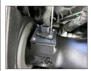
21. Install the Driver side and passenger side intake tubes into the vehicle. Remove the MAF sensors from the stock air boxes and install into the new K&N tubes and secure using provided hardware. Note: Arrow on the MAF sensors will go in direction towards throttle body.
