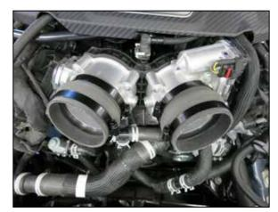
18. Install the hump hoses with clamps provided to the throttle body.
