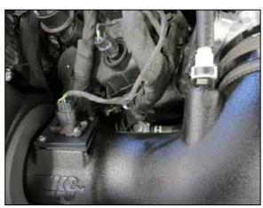
22: Reconnect the MAF sensor harness on passenger side and connect the EVAP line to
