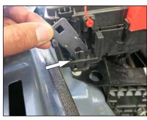
12. Using a smaller flathead screwdriver.Lift the tab from the bottom and remove the metal tab from the fuse box. Set the Relay harness off to the side.
