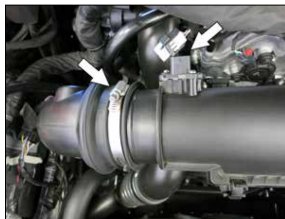
2. Disconnect the MAF sensor electrical connection and then loosen the hose clamp that secures the factory intake tube to the remove air filter housing.
