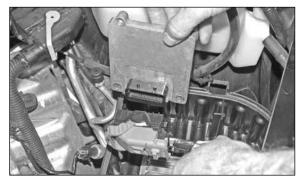
9. Remove the transmission control module from the housing, release the clamshell retaining clip, and then disconnect the wiring harness as shown.
