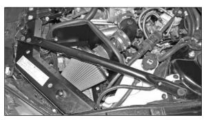
39. Reinstall the body brace removed in step #6 and secure with the factory bolts.
