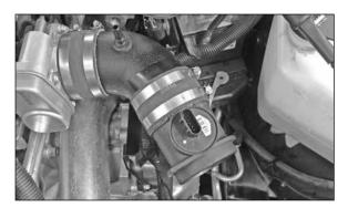
27. Install the mass air sensor assembly onto the  $K\&N^{\odot}$  intake tube as shown and secure with the provided hose clamp.
