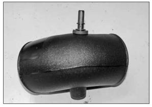
24. Install the factory crank case vent fitting removed in step #20 into the grommet installed into the K&N<sup>®</sup> intake tube in step #19.
