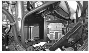
34. Place the engine control module assembly into position on top of the heat shield, then secure the heat shield and control module bracket to the inserted nuts installed in step #31 with the provided hardware.
