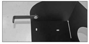
28. Install the mounting bracket (070952) onto the heat shield with the provided hardware.
