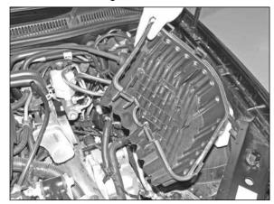
12. Pull up the lower air box housing to release it from the mounting grommets and then remove the housing from the vehicle as shown.
