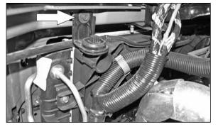
32. Remove the top left radiator mounting bracket bolt shown.
