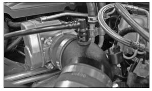
40. Reconnect the crank case vent tube to the vent fitting as shown.
