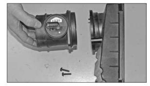
22. Remove the two screws, which secure the mass air sensor to the air filter housing and then remove the mass air sensor as shown.
