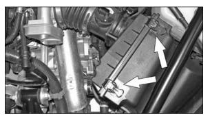
4. Loosen the hose clamp, which secures the intake tube to the throttle body, and release the air box over center clips shown.
