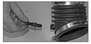
20. Remove the crank case vent fitting from the stock intake tube as shown. **NOTE: This fitting will be reused.**  25. Install the K&N<sup>®</sup> intake tube into the silicone hose at the throttle body and align with the mounting bracket installed in step #17. Secure the silicone hose onto the throttle body with the supplied hardware and hose clamp. **NOTE: Do not completely tighten at this time.**
