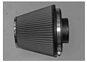
36. Install the filter adapter into the K&N<sup>®</sup> air filter as shown and secure with the provided hardware.
