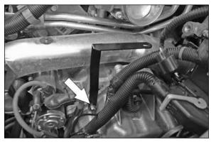
17. Install the tube mounting bracket (26627) onto the existing transmission stud as shown. **NOTE: It will be necessary to remove the wiring harness retaining clip from the stud.**
