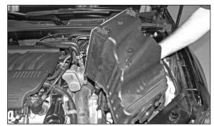
2. Depress the locking tab on the mass air sensor electrical connection, then disconnect the mass air sensor electrical connection as shown.
