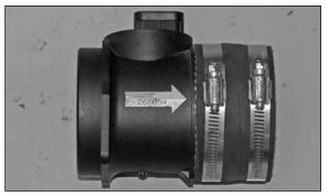
26. Install the silicone hose (08690) onto the mass air sensor as shown and secure with the provided hose clamps.
