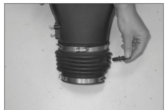
9. Remove the crank case vent fitting from the stock intake tube as shown.
