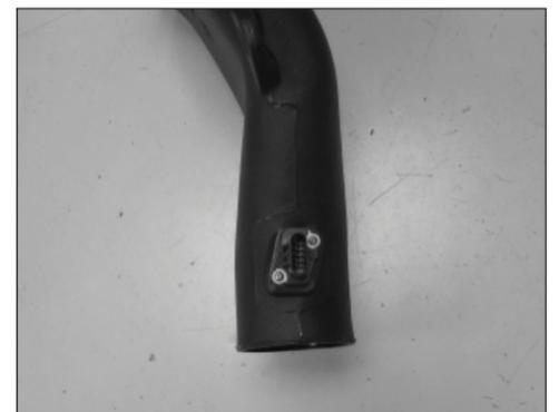
8. Secure the mass air sensor to the K&N Intake Tube with the screws and spacers provided.
