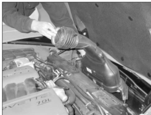
5. Pull the intake tube off of the throttle body and dislodge the intake tube from the mounting pins on the radiator cover. Then remove the complete intake assembly from the vehicle.
