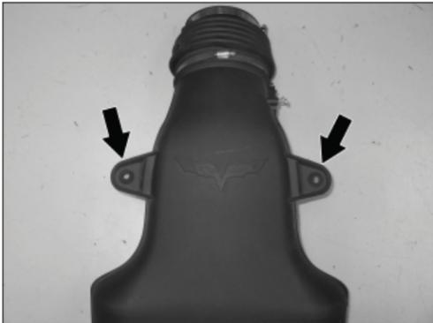
12. Remove the two mounting grommets shown from the stock intake tube.
