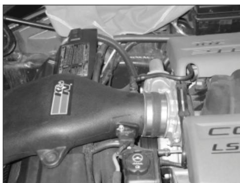
18. Install the K&N intake assembly onto the mounting pins and into the silicone hose at the throttle body and secure with the provided hose clamp and then reconnect the crank case vent hose.
