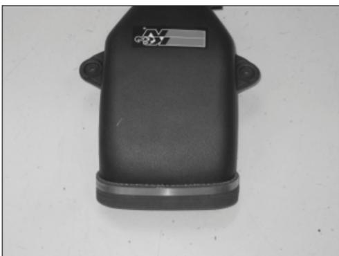
14. Install the supplied silicone hose (08619) onto the K&N Intake Tube and secure with the supplied hose clamp. **NOTE: Be sure to place the notches in the silicone hose over the air diverter mounting bolts.**
