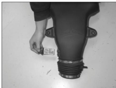
6. Remove the two screws which secure the mass air sensor in the stock intake tube and then remove the sensor as shown.
