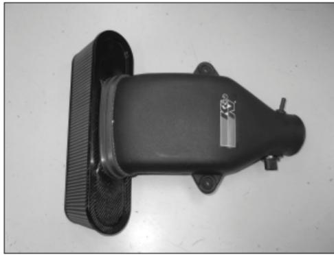
15. Install the K&N Air Filter into the silicone hose installed on the K&N Intake Tube as shown and secure with the provided hose clamp.
