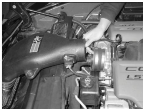
17. Install the K&N intake assembly into position and connect the mass air sensor electrical connection.
