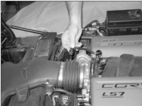
2. Unlock and disconnect the crank case vent hose from the intake tube as shown.
