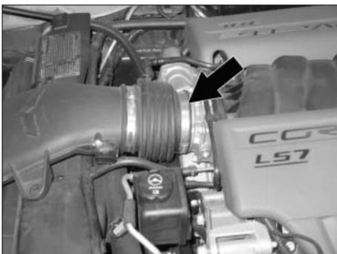
4. Loosen the hose clamp that secures the intake tube to the engine throttle body.
