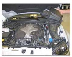
7. Pull up firmly and remove the air box from the
