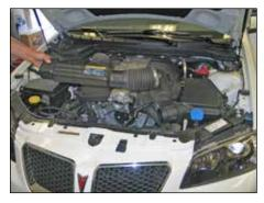
Remove the intake tube from the vehicle
