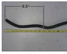
24. Measure 8.5' from the end of the tube and then cut the tube using a sharp knife.
