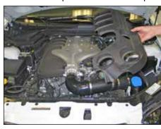
21. Remove the driver's side engine cover as shown.
