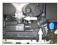
4. Loosen the hose clamps which secure the factory intake tube to the mass air sensor and throttle body.
