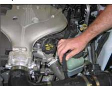
26. Install the crank case breather hose onto the valve cover and connect the open end to the vent fitting attached to the K&N® intake tube.
