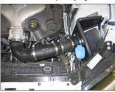
20. Install the intake tube assembly onto the throttle body and mass air sensor, adjust for proper fit then secure with the provided hose clamps.
