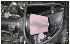
25. Install the K&N<sup>®</sup> air filter onto the filter adapter and secure with the provided hose clamp. NOTE: Drycharger<sup>®</sup> air filter wrap; part # RF-1042DK is available to purchase separately. To learn more about Drycharger<sup>®</sup> filter wraps or look up color availability please visit http://www.knfilters.com<sup>®</sup>.
