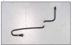
24a. On 2014 and later vehicles, it will be necessary to cut the crank case vent tube as shown. Then connect the cut section of tube to the oil filler cap. Attach the supplied hose to the to the trimmed section of crank case vent tube,
