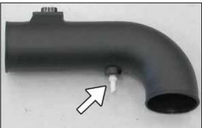
22. Install the provided 1/4 NPT fitting into the  $K\&N^{\ensuremath{\circledast}}$  intake tube as shown. NOTE: Plastic NPT fittings are easy to cross thread. Install the vent fitting "hand" tight, then turn it two complete turns with a wrench.
