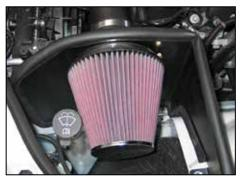
23. Install the  $K\&N^{\otimes}$  air filter and secure with the provided hose clamp.
