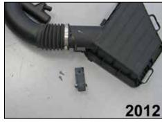
17. Remove the two screws that secure the mass air sensor into the factory intake tube.
