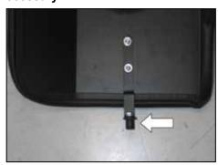
12. Install the provided inserted nut onto the heat shield mounting bracket and secure with the provided hardware.
