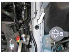
8. Remove the air box mounting grommet shown on the frame rail.
