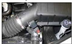
3. Slide the red locking tab back and then disconnect the mass air sensor electrical connection.
