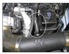
22. Remove the 90° vent hose from the crank case vent tube. Install the provided silicone vent hose and install it onto the fitting installed into the K&N® intake tube. Trim the vent hose for proper fit.
