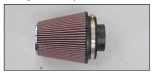
10. Install the filter adapter into the K&N® air filter and secure with the provided hose clamp
