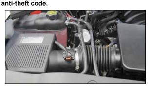
2. Disconnect the mass air sensor electrical connection and unhook the wiring harness from the air filter housing.
