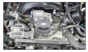
12. Install the provided step hose (084055) onto the throttle body and secure with the provided hose clamp.
