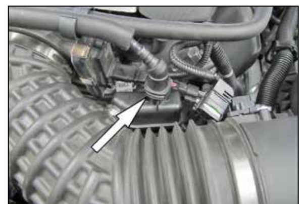
3. Disconnect the crank case vent quick connect fitting from the intake tube.
