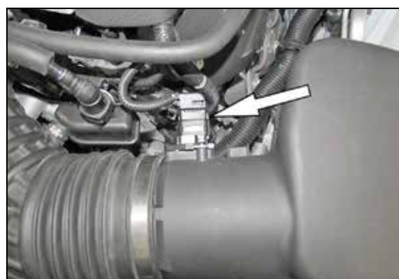
2. Disconnect the mass air sensor electrical connection.
