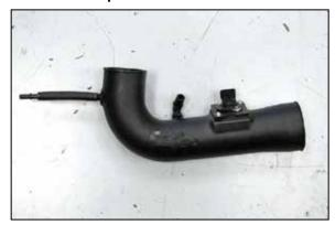
25. Install the 90° crank case vent fitting into the  $K\&N^{\otimes}$  intake tube as shown.
