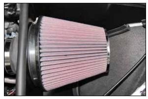
30. Install the K&N<sup>®</sup> air filter and secure with the provided hose clamp.
