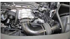
17. Install the intake tube assembly into the hump coupler and then into the coupler at the throttle body, adjust the tube for best fit and then secure
