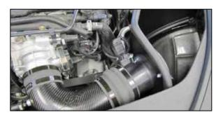
19. Connect the mass air sensor electrical connection.
