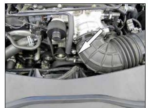
4. Disconnect the crank case vent quick disconnect
