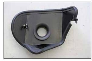
8. Install the edge trim onto the heat shield as shown. Some trimming of the edge trim will be necessary.
