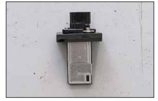
15. Install the mass air sensor into the K&N<sup>®</sup> mass air sensor adapter and secure with the provided hardware.
