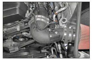
18. Install the Intake tube into the coupler at the filter adapter and then into the coupler at the turbo inlet chamber, adjust the tube and heat shield for best fit and then secure with the provided hose clamps. Reconnect the mass air sensor electrical connection and secure the wiring harness to the insert in the intake tube.
