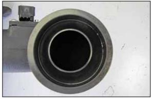
17. Install the air diffuser into the K&N<sup>®</sup> intake tube so the radiused surface is located inside the tube.
