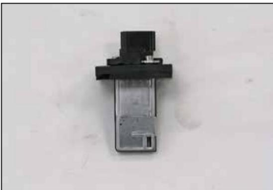
11. Remove the mass air sensor from the factory air filter housing. Install the sensor and provided gasket onto the K&N® filter adapter as shown.
