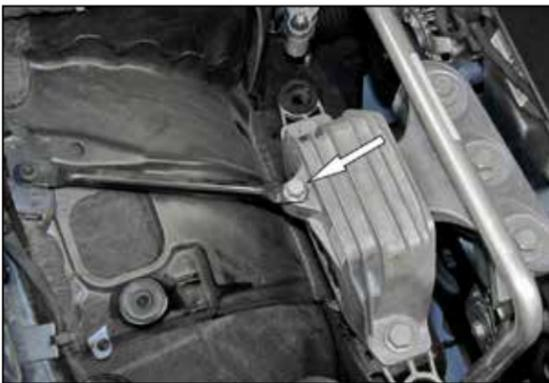
9. Remove the bolt shown from the fender brace.
