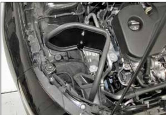
10. Install the heat shield into position and secure with the bolt removed in the previous step.
