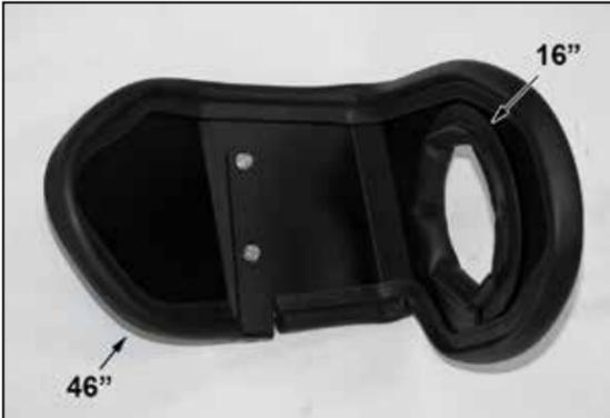
8. Install the 16" section into the heat shield and the 46" section around the heat shield as shown.
