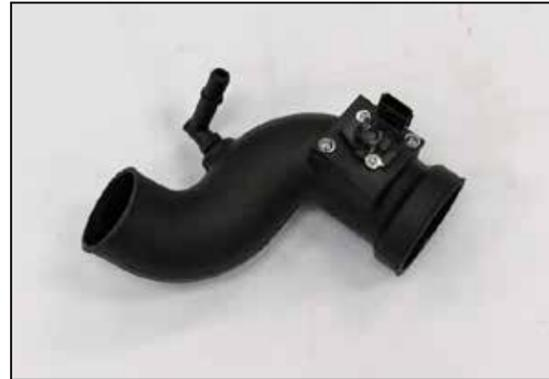
13. Install the provided quick disconnect fitting into the K&N® intake tube as shown.
