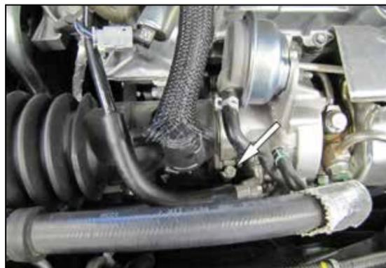
4. Loosen the hose clamp that secures the intake tube to the turbo inlet then disconnect the tube from the turbo. Lift the intake assembly up to dislodge it from the mounting grommets and then remove the complete intake system from the vehicle.
