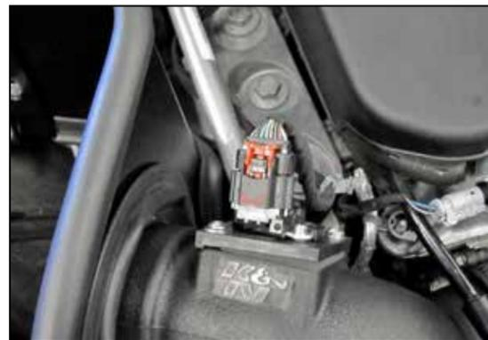
16. Connect the mass air sensor electrical connection.
