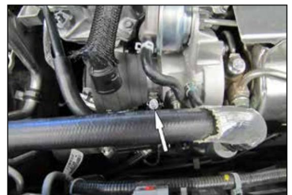
5. Install the provided coupler (5-1045) onto the turbo inlet and secure with the provided hose clamp.
