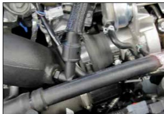
15. Connect the CCV hose to the quick disconnect fitting installed into the K&N® intake tube.
