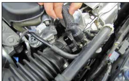
3. Snap the provided quick release tool onto the CCV tube, then push it up to unlock the CCV quick release connector and disconnect the CCV hose from the intake tube.
