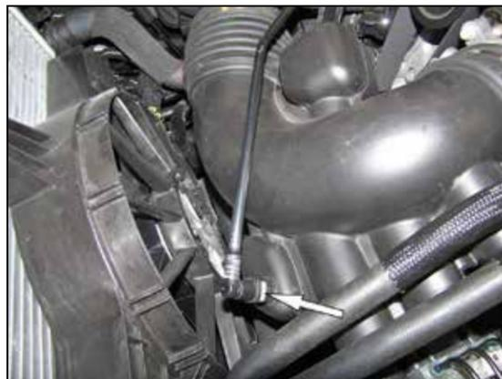
4. Release the locking tab and then disconnect the crank case vent line from the factory intake tube.
