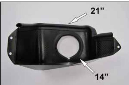
12. Install the edge trim onto the K&N® heat shield as shown.
