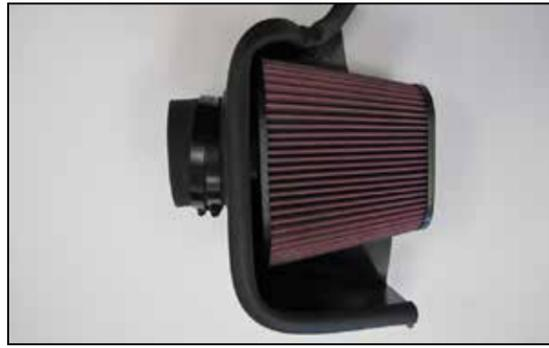
13. Install the K&N® air filter into the heat shield, install coupler hose (08761) onto the filter and secure with the provided hose clamp.
