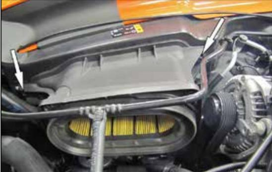
8. Remove the two bolts that secure the air filter housing to the inner fender and then remove the housing and air filter from the vehicle.
