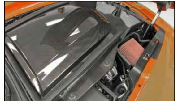
22. Reinstall the super charger cover and secure with the factory hardware.
