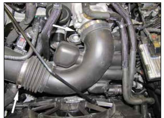
5. Loosen the two hose clamps that secure the factory intake tube and then remove the intake tube from the vehicle.
