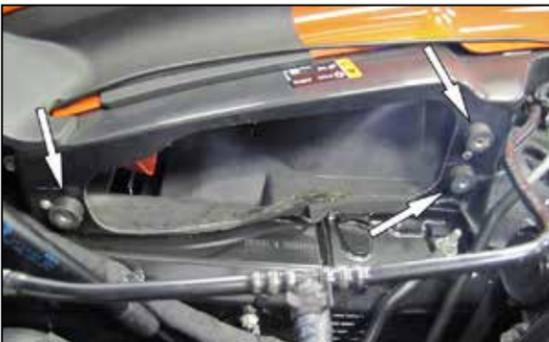
10. Install the three rubber mounted studs into the air filter housing mounting location as shown.
