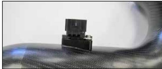
16. Remove the mass air sensor from the factory mass air sensor housing and install it into the K&N® intake tube using the provided hardware.
