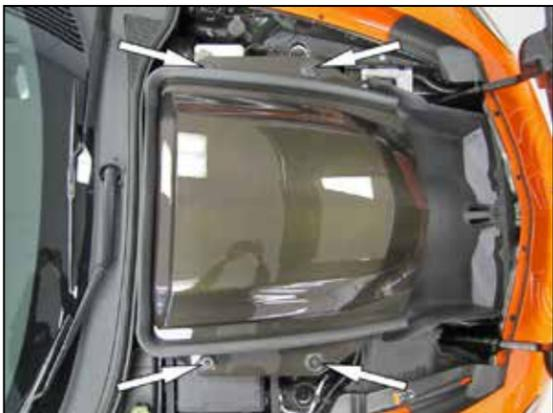
2. Loosen the four bolts that secure the supercharger cover, remove the bolts and then remove the cover from the vehicle.
