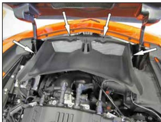
3. Loosen the four bolts that secure the air extractor duct to the radiator and then remove the extractor from the vehicle.
