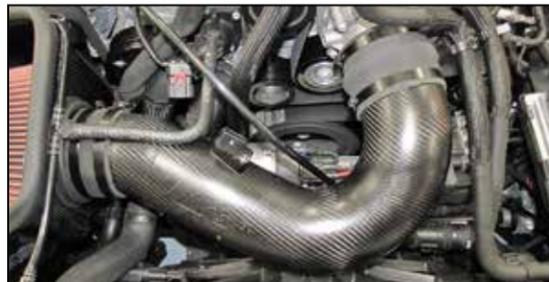
18. Install the K&N® intake tube into the coupler hose at the air filter and then into the coupler at the throttle body. Adjust the tube for best fit and then secure with the provided hose clamps.
