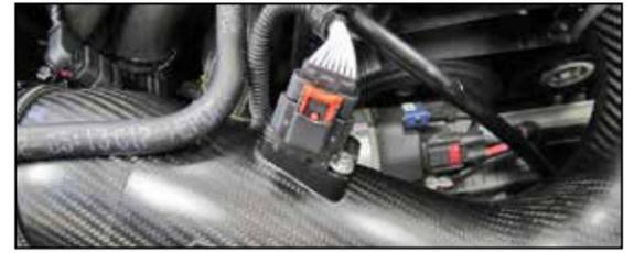
20. Using the provided extension harness, reconnect the mass air sensor electrical connection.
