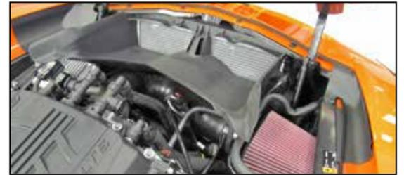
21. Reinstall the air extractor duct and secure with the factory hardware.
