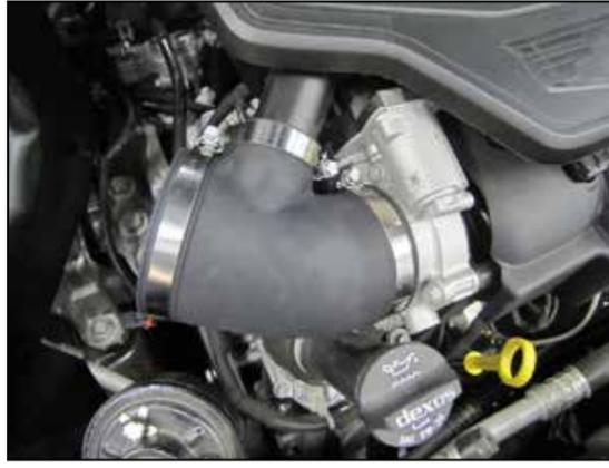
10. Install the provided coupler onto the throttle body and intake plenum. Secure with the provided hose clamps.
