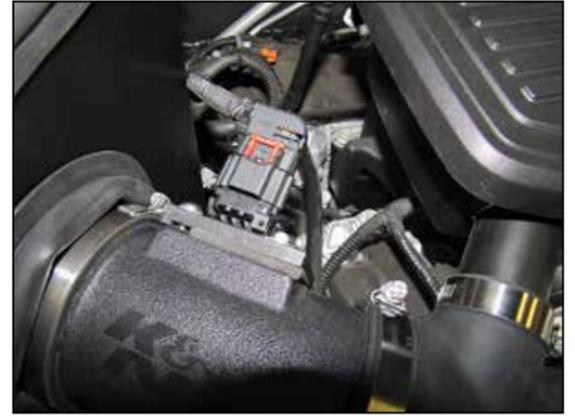
14. Reconnect the mass air sensor electrical connection.
