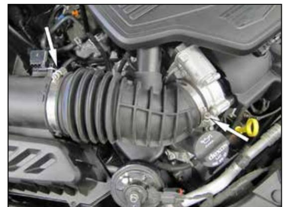
4. Loosen the two hose clamps that secure the factory intake hose. Remove the factory intake hose from the vehicle.
