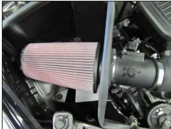
13. Install the air filter onto the intake tube, adjust the intake tube and filter for best fit and then secure the hose clamp.
