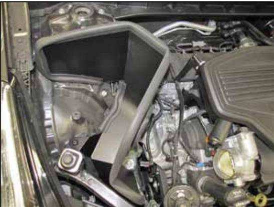
9. Install the heat shield assembly into the vehicle.
