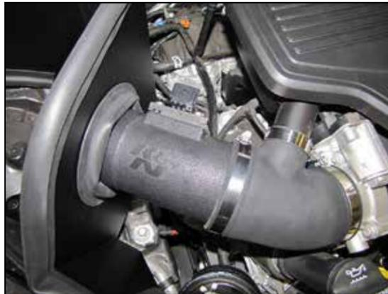
12. Install the K&N® intake tube assembly into the heat shield and coupler.
